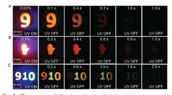
Fig. 6 Photographs of afterglow objects with desired shapes prepared by melt casting technique of (A) NPhRedBF2-MeOBP-0.01%, (B) NPhRedBF2-MeOBP-0.1% and (C) (left-right) NPhRedBF2-MeOBP-0.01%, N $\alpha$ N-MeOBP-0.5% and N $\beta$ NBF $_2$ -MeOBP-0.5% under 365 nm UV light and after removal of the UV light.
