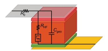
Fig. 6 Schematic with series resistance  $R_0$ , high-frequency resistance  $R_{\rm HF}$ , and a potential LF feature. Grey and yellow rectangles represent the current collectors, and the brown, red and green layers represent the absorber and transport layers, respectively.
