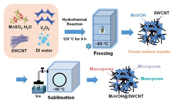
Fig. 1 Schematic illustration of the freeze-drying process utilized to achieve the different pore-sized structures for pristine MnVOH and the MnVOH@SWCNT nanocomposite.
