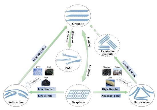
Fig. 1 Schematic diagram of the structural evolution of different pure carbon materials: graphite can be transformed into graphene or rGO by physical or chemical methods; soft carbon can be obtained from PVC, coal, pitch, etc. after graphitization at high temperature, soft carbon can be transformed into artificial graphite; hard carbon is mostly obtained from biomass, and can be transformed into crystallite graphite after graphitization.
