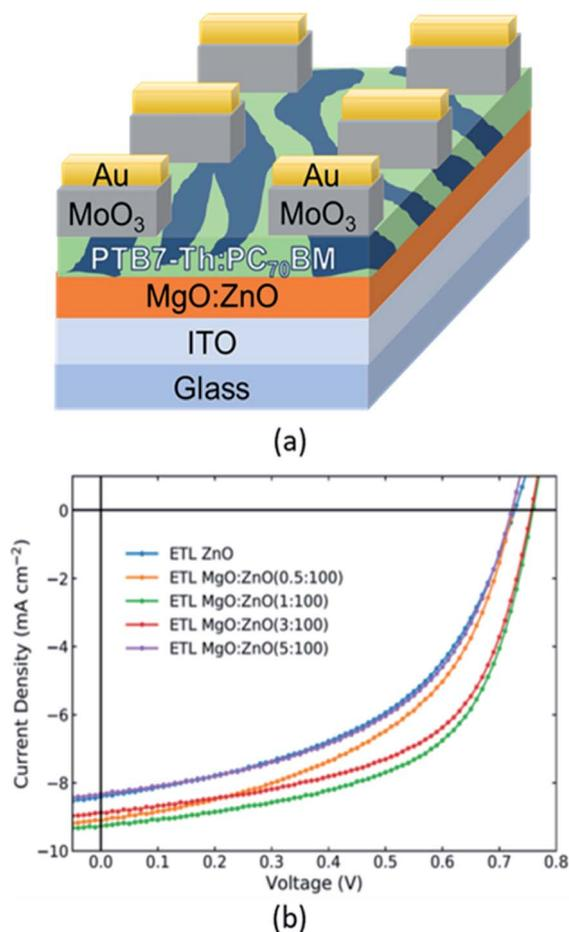
**Fig. 1** (a) Schematic of the multi-layered structure of the OPV device. 5 Types of OPVs were tested, 4 with ETLs containing different amounts of Mg-doping in ZnO and an undoped “control” device. (b) Representative current density vs. voltage curves under 1 sun. Corresponding average key performance indicators from 8 distinct devices for each type of ETL are reported in Table 2.
