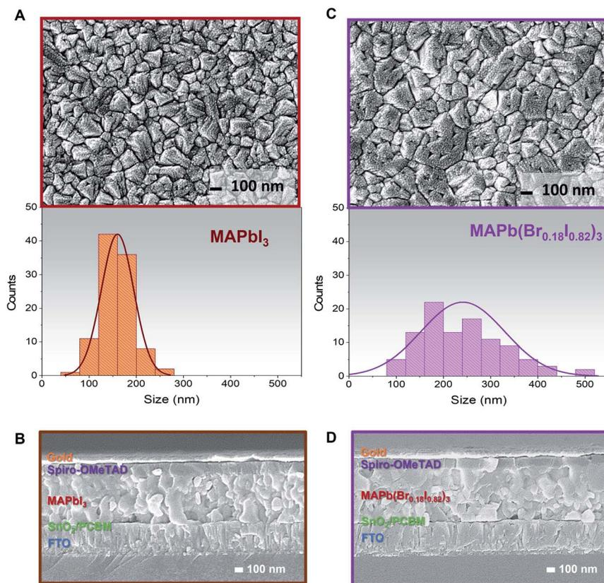
Fig. 3 MAPbI<sub>3</sub> and MAPb(Br<sub>0.18</sub>I<sub>0.82</sub>)<sub>3</sub> FESEM images. Top view, grain size distribution histogram (obtained over 100 grains), and cross-section FESEM images of (A and B) MAPbI<sub>3</sub> (brown) and (C and D) MAPb(Br<sub>0.18</sub>I<sub>0.82</sub>)<sub>3</sub> (purple).
