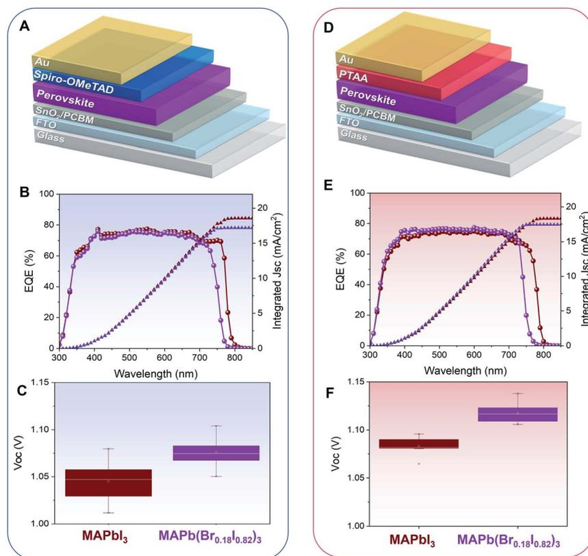
Fig. 5 MAPbI<sub>3</sub> and MAPb(Br<sub>0.18</sub>I<sub>0.82</sub>)<sub>3</sub> perovskite solar cells (PSCs) (A) schematic of n-i-p PSCs with Spiro-OMeTAD as HMT, (B) EQE, (C) V<sub>oc</sub> for MAPbI<sub>3</sub> and MAPb(Br<sub>0.18</sub>I<sub>0.82</sub>)<sub>3</sub>. (D) Schematic of n-i-p PSCs with PTAA as HMT, (E) EQE, (F) V<sub>oc</sub> for MAPbI<sub>3</sub> and MAPb(Br<sub>0.18</sub>I<sub>0.82</sub>)<sub>3</sub>.
