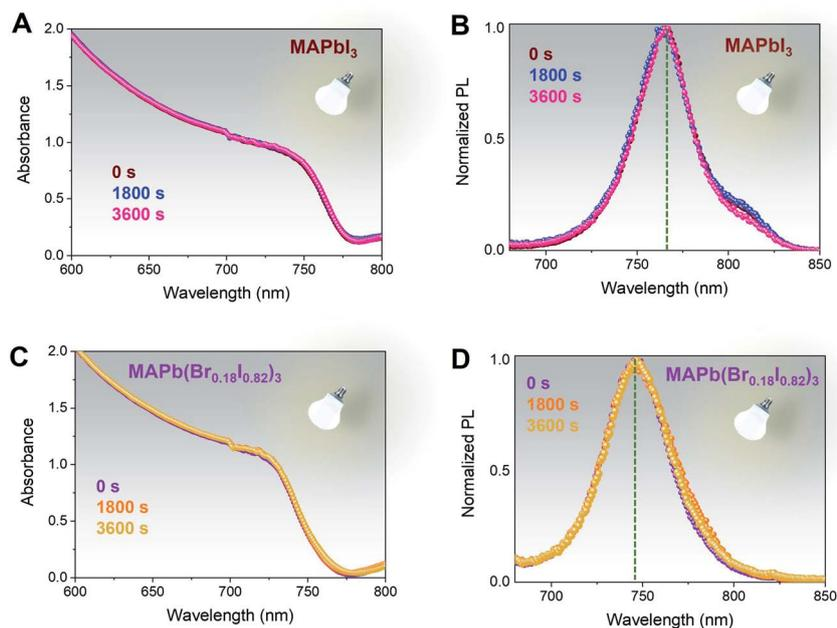
Fig. 4 MAPbI<sub>3</sub> and MAPb(Br<sub>0.18</sub>I<sub>0.82</sub>)<sub>3</sub> light stability. UV-vis absorbance and photoluminescence spectra under continuous 1 sun illumination for over 3600 s for (A and B) MAPbI<sub>3</sub> and (C and D) MAPb(Br<sub>0.18</sub>I<sub>0.82</sub>)<sub>3</sub>.
