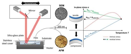
Fig. 6 (Left) Scheme of the setup of the thin film stress instrument used for curvature determination. It has a built-in heater for *in situ* measurements. (Right) Temperature dependence of the in-plane stress while heating (red dotted line) and the following natural cooling process (straight arrows). The different thermal expansion coefficients of the film and substrate directly affect the resulting residual stress. Rearranged with permission from ref. 57.
