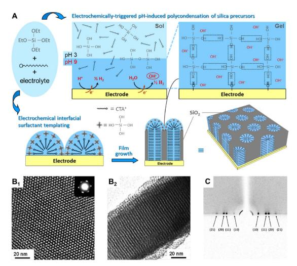
Fig. 3 (A) Schematic illustration of the EASA process. (B) TEM images of the ordered and oriented mesoporous silica film (B<sub>1</sub> top view with electron diffraction pattern as inset; B2 cross-section). (C) Typical GI-XD pattern confirming the hexagonal packing of vertically aligned mesopore channels. Reproduced with permission from ref. 40.
