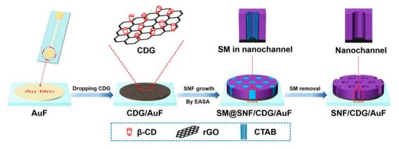
Fig. 12 Illustration of facile preparation of silica nanochannel array film (SNF)/B-cyclodextrin-graphene (CDG)/AuF by EASA method using CDG as nanoadhesive. SM = surfactant micelle. Reproduced with permission from ref. 92.
