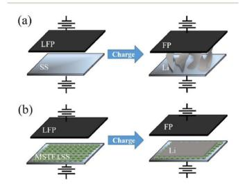
Fig. 10 Schematic illustrations of the Li electrodeposition process on the (a) stainless steel (SS) and (b) mesoporous silica thin films with channels perpendicular to the stainless steel substrate (MSTF $\perp$ SS) in the anode-free Li metal batteries. Reproduced with permission from ref. 79.
