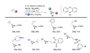
Scheme 31 Electrochemical synthesis of aziridines from alkenyl thianthrenium salts.
