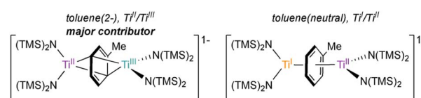
Fig. 3 Electronic representation of 6-K as either Ti II /Ti III bridged by a toluene dianion (left) or Ti I /Ti II bridged by a neutral toluene (right).
