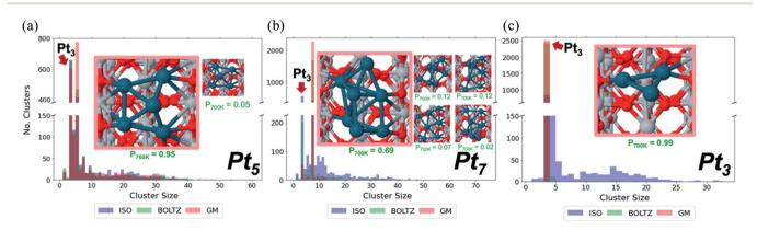
Fig. 6 Sintering outcomes of fluxional size-selected Pt clusters, as demonstrated by histograms of final cluster size distribution, of sizes (a) Pt<sub>5</sub>, (b) Pt<sub>7</sub>, and (c) Pt<sub>3</sub> on rutile. Each cluster size responds differently to level of isomeric diversity of the starting point.
