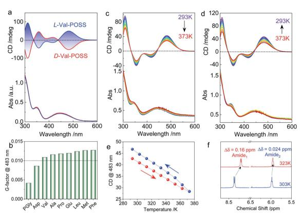
Fig. 3 (a) CD spectra of Val-POSS in CHCl<sub>3</sub> (1 mM) with different configurations. (b) Dissymmetry g-factors of different building units, "POSS" was omitted for clarity. (c-e) Temperature-variable CD spectra with heating and cooling processes of Val-POSS (1 mM in dioxane). (f) Partial <sup>1</sup>H NMR spectra of Val-POSS in CDCl<sub>3</sub> at different temperatures.
