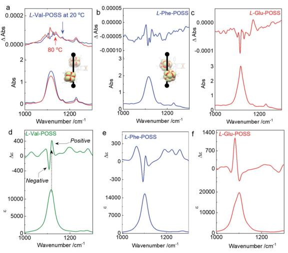
Fig. 4 (a–c) VCD spectra of Val-POSS, Phe-POSS and Glu-POSS in  $CCl_4$  (50 mg mL<sup>-1</sup>) respectively. Insets display the corresponding intramolecular folding of POSS segments. (d–f) Calculated VCD spectra of Val-POSS, Phe-POSS and Glu-POSS respectively *via* time-dependent DFT (TDDFT) at B3LYP/6-31g(d) level of theory (full width at half maximum = 15 cm<sup>-1</sup>).
