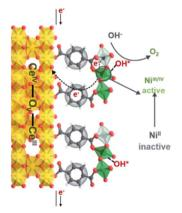
Fig. 5 Schematic illustration of possible electron transfer paths occurring in the  $CeO_2$ @NiFe-MOF heterostructures under electrocatalysis processes for the OER catalysis.
