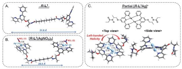
Fig. 7 DFT-optimized structures; (A)  $R-L^1$ , (B)  $[R-L^1(AgNO_3)_2]$  and (C) partial  $[R-L^1Ag]^+$  viewed from the side and top. The local coordination geometry and bond lengths are displayed.
