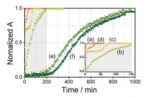
Fig. 4 Time-dependent UV-Vis spectral changes of R-L<sup>1</sup> (7.2 mM) with AgNO<sub>3</sub> in a mixture of H<sub>2</sub>O and DMSO (1 : 1 v/v); (a) 0 equiv., (b) 0.4 equiv., (c) 0.6 equiv., (d) 0.8 equiv., (e) 1.2 equiv., and (f) 1.4 equiv.
