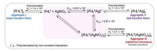
Fig. 5 Proposed chiral self-sorting supramolecular polymerization of  $R-L^1$  at different concentrations of AgNO<sub>3</sub> (the formation of aggregate II with left-helicity). The stability constants ( $K_{1Ag}$  and  $K_{2Ag}$ ) were determined by UV-Vis titration using a previously reported method.<sup>48–50</sup>
