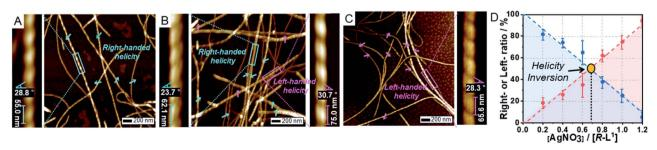
Fig. 2 AFM images of self-assembled  $R-L^1$  with AgNO<sub>3</sub> obtained in a DMSO and H<sub>2</sub>O mixture (1 : 1 v/v): (A) 0.0, (B) 0.2, and (C) 1.2 equiv. (D) Plot of the ratio of right- or left-handed helical fibers vs. equivalents of AgNO<sub>3</sub>. The ratio of right- to left-handed fiber was calculated by the number of individual fibers (50–100); the blue and the red colors indicate the ratio of right- and left-handed fibers, respectively.
