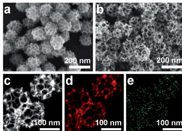
Fig. 2 (a and b) SEM images of the obtained products (a) before and (b) after HCl etching treatment. (c–e) HAADF-STEM image and corresponding elemental maps (Pd (red) and Bi (green)).
