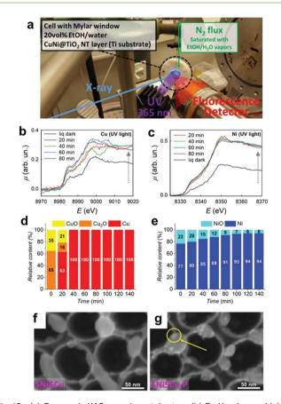
Fig. 13 (a) Operando XAS experimental setup; (b) Cu K-edge and (c) Ni K-edge XAS spectra of 5Ni5Cu-TiO<sub>2</sub> in a water—ethanol under UV irradiation for various exposure times; (d) Cu and (e) Ni phase contents determined by operando XAS for 5Ni5Cu-TiO<sub>2</sub>; SEM images of 5Ni5Cu-TiO<sub>2</sub> (f) before and (g) after photocatalysis (a yellow circle indicates metallic NPs deposited under the UV irradiation). Adapted with permission from ref. 171; copyright 2020 ACS.
