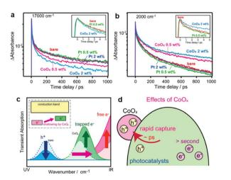
Fig. 10 Decay of transient absorption at (a) 17 000 cm $^{-1}$  and (b) 2000 cm $^{-1}$  for bare, CoO $_x$ -loaded, and Pt-loaded LaTiO $_2$ N after excited by 500 nm laser pulses; (c and d) schematics showing the change in carrier dynamics upon CoO $_x$  CC loading. Adapted with permission from ref. 157; copyright 2014 ACS.
