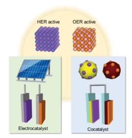
Fig. 1 Application of materials active for solar-driven water splitting *via* the hydrogen evolution reaction (HER) and oxygen evolution reaction (OER).
