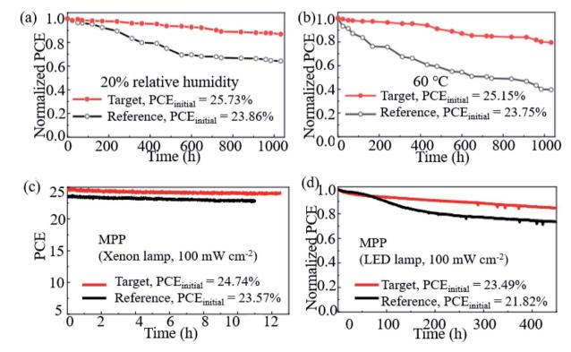
Fig. 10 Stability of the FAPbI<sub>3</sub> PSCs. (a) Shelf-life stability of the reference (FAPbI<sub>3</sub>) and target (FAPbI<sub>3</sub> with 2% FAHCOO additive) PSCs. (b) Heat stability of the reference and target PSCs. (c) Operational stability of the reference and target PSCs. (d) Long-term operational stability of the reference and target PSCs. Reprinted with permission from ref. 31, copyright 2021, Nature Publishing Group.
