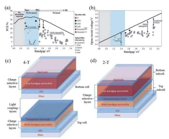
Fig. 7 (a) Shockley–Queisser efficiency and (b) calculated maximum  $V_{\rm OC}$  (radiative limit). Reprinted with permission from ref. 32, copyright 2017, Science Publishing Group. Structure diagram of (c) 4-T and (d) 2-T solar cells. Reprinted with permission from ref. 96, copyright 2019, Advanced Functional Materials.
