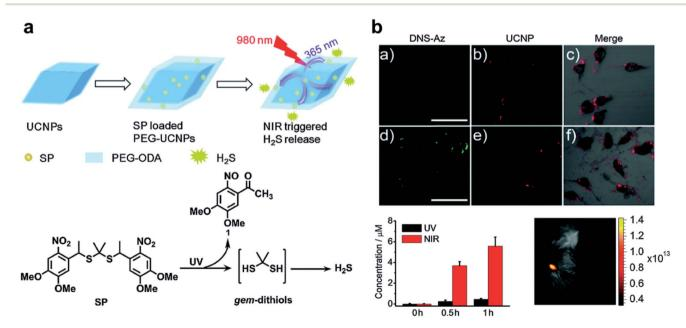
$\textbf{Fig. 6} \quad \text{UCNP-based nanocomposites for $H_2$S gas therapy. (a) Construction of $P$-loaded PEG-UCNPs platform for NIR-triggered $H_2$S release. (b) }$ H<sub>2</sub>S release from SP-loaded PEG-UCNPs with laser irradiation.<sup>38</sup> Adapted from ref. 38 with permission from Royal Society of Chemistry, copyright 2015.
