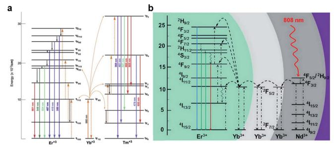
Fig. 1 Proposed energy transfer mechanism showing the UCL processes in (a) Er<sup>3+</sup>, Tm<sup>3+</sup>, and Yb<sup>3+</sup> doped UCNPs under 980 nm laser excitation31 and (b) Nd3+, Yb3+, and Er3+ doped UCNPs under 808 nm laser excitation32 Adapted from ref. 31 with permission from Elsevier Ltd, copyright 2014; adapted from ref. 32 with permission from American Chemical Society, copyright 2016.
