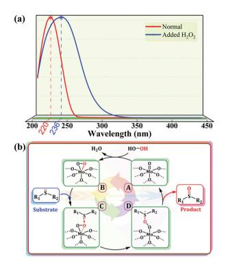
Fig. 7 (a) UV-vis spectra of 1 before and after treatment with H<sub>2</sub>O<sub>2</sub>. (b) A mechanistic diagram of MPS or CEES oxidation.
