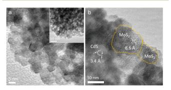
Fig. 2 Representative (a) TEM and (b) HRTEM images of the  $20\text{-MoS}_2/\text{CdS}$  NCAs catalyst.
