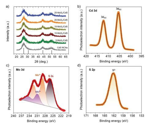
Fig. 1 (a) XRD plots for the mesoporous CdS and  $MoS_2/CdS$  NCAs. The standard diffraction data of the zinc blende CdS according to the JCPDS card no. 42-1411 are also shown (black bars). (b-d) Typical XPS core-level spectra of the Cd 3d (b), Mo 3d (c) and S 2p (d) region for the 20- $MoS_2/CdS$  catalyst.
