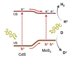
Scheme 1 Expected charge transfer during photocatalytic H<sub>2</sub> production on mesoporous MoS<sub>2</sub>/CdS NCAs under visible light excitation.
