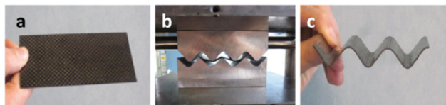
Fig. 3 Thermoforming of a cured composite laminate. A 2 mm thick carbon fibre reinforced dynamic epoxy laminate (a) was compression-moulded in a zig-zag shaped mould (b), rendering a thermoformed way 3D part (c). Reproduced with permission from ref. 43. Copyright 2016 Royal Society of Chemistry.
