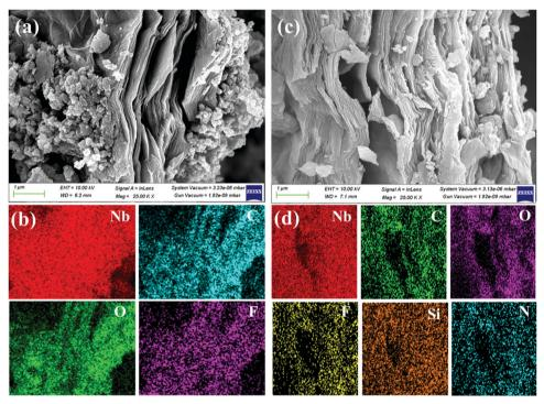
FESEM and the corresponding elemental mapping of pristine  $Nb_2CT_x$  MXene (a and b) and  $Nb_2CT_x$ -0.2 ApTES MXene (c and d)
