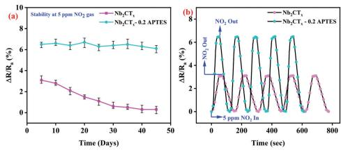
Fig. 8 (a) Long-term stability and (b) repeatability of Nb<sub>2</sub>CT<sub>x</sub> and Nb<sub>2</sub>CT<sub>x</sub>-0.2 APTES-based NO<sub>2</sub> gas sensor.
