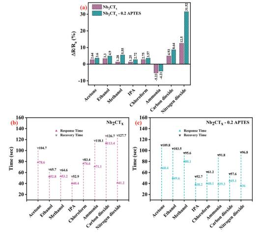
Fig. 7 (a) Selectivity of Nb<sub>2</sub>CT<sub>x</sub> and Nb<sub>2</sub>CT<sub>x</sub>-0.2 APTES based sensor and (b and c) their response–recovery time to different analytes.
