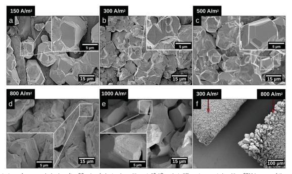
Fig. 2 Substrate surface morphologies after 20 min of electrodeposition at 40 °C and at different current densities. SEM images of the center of the substrate after electrodeposited at current densities of (a) 150 A m<sup>-2</sup>, (b) 300 A m<sup>-2</sup>, (c) 500 A m<sup>-2</sup>, (d) 800 A m<sup>-2</sup>, and (e) 1000 A m<sup>-2</sup> and (f) the corner of the substrate after electrodeposition at current densities of 300 A m<sup>-2</sup> (left) and 800 A m<sup>-2</sup> (right).
