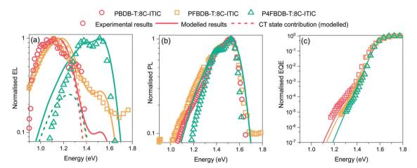
Fig. 3 Steady state optical properties of the blends. (a) Normalised electroluminescence spectra of the three blend devices at an injection current of 100 mA cm<sup>-2</sup>. (b) Normalised Photoluminescence spectra of the devices. (c) Normalised EQE of the three blends. Solid lines show the model results.
