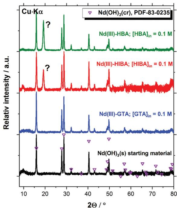
Fig. 9 XRD patterns of the Nd(III) solid phase used as starting material, and the corresponding solid phases after equilibration in the solubility experiments with GTA, HIBA and HBA at  $[L]_{\text{tot}} = 0.1$  M. Symbols reproduce the patterns reported for  $\text{Nd}(\text{OH})_3(\text{cr})$  (PDF-83-0235) reference material.
