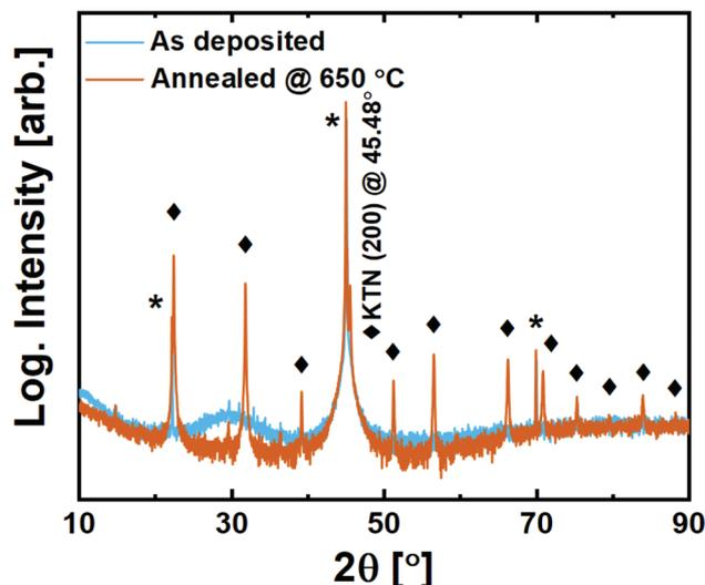
Fig. 10 X-ray diffraction of 200 nm  $\text{KTa}_{0.67}\text{Nb}_{0.35}\text{O}_3$  thin films deposited on  $\text{MgAl}_2\text{O}_4$  (100) substrates. Substrate reflections are marked with \*, while perovskite film reflections are marked with ◆.
