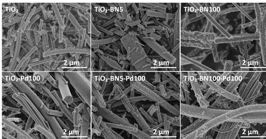
Fig. 2 SEM images of TiO<sub>2</sub>, TiO<sub>2</sub>-BN5, TiO<sub>2</sub>-BN100, TiO<sub>2</sub>-Pd100, TiO<sub>2</sub>-BN5-Pd100 and TiO<sub>2</sub>-BN100-Pd100 nanocomposites.
