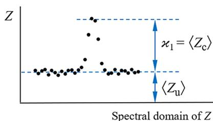
Fig. 2 How to separate the first cumulant from the uncorrelated background. Cumulant  $\kappa_1$  measures only the correlated fragments  $Z_c$  that form a peak on a spectrum. The peak rides on a background of uncorrelated fragments  $Z_u$ . This definition of  $\kappa_1$  keeps the background parameter  $\zeta_z = \langle Z_u \rangle / \langle Z_c \rangle$  consistent with the higher cumulants.
