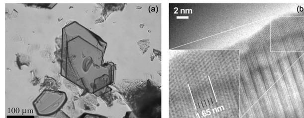
**Fig. 10** (a) Optical image of single crystals of InFeO<sub>3</sub>(ZnO)<sub>4</sub>. (b) HRTEM images of InFeO<sub>3</sub>(ZnO)<sub>4</sub> imaged along *<2110>* zone axis. Dark spot lines have the In-layer spacing of 1.65 nm. Panels (a and b) are reprinted with permission from ref. 54. © 2014 John Wiley and Sons, Inc.
