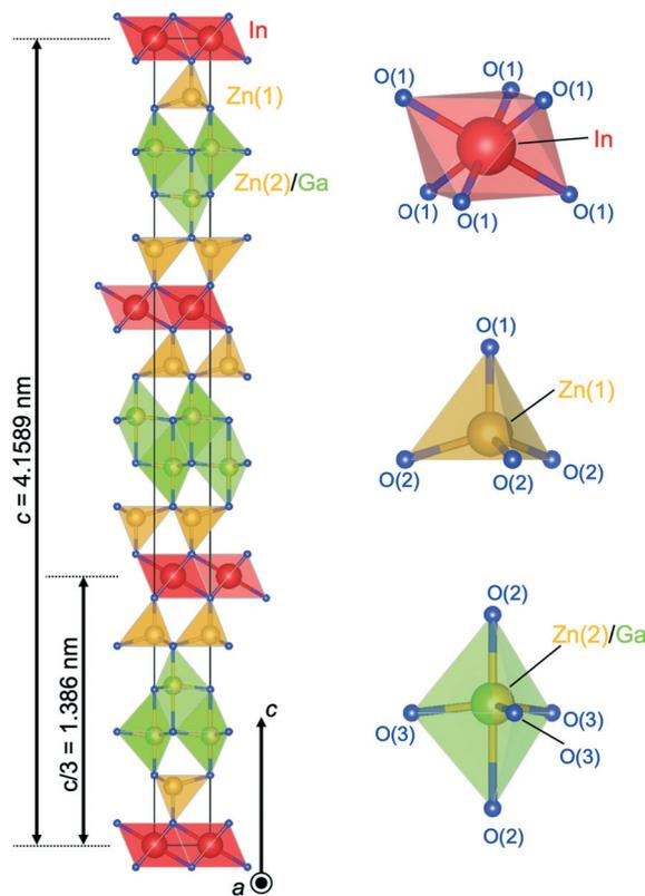
Fig. 6 Crystal structure of  $\text{InGaO}_3(\text{ZnO})_3$ . Coordination of  $\text{InO}_6$  is octahedra,  $\text{Zn}(1)\text{O}_4$  is tetrahedra, and  $\text{Zn}(2)/\text{GaO}_5$  is trigonal bipyramid.
