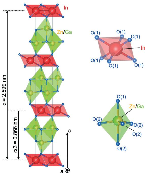
Fig. 5 Crystal structure of  $\text{InGaO}_3(\text{ZnO})_1$ . Coordination of  $\text{InO}_6$  is octahedra and  $\text{Zn/GaO}_5$  is trigonal bipyramid. Because Zn and Ga cannot be separated, the Zn/Ga mixed site is referred to as the trigonal bipyramid in this paper.
