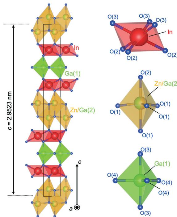
**Fig. 17** Crystal structure of  $(\text{InGaO}_3)_2\text{ZnO}$ . Coordination of  $\text{InO}_6$  is octahedra,  $\text{Zn/Ga(2)O}_5$  trigonal bipyramids (two  $\text{Zn/Ga(2)O}_4$  tetrahedra), and  $\text{Ga(1)O}_5$  trigonal bipyramid.
