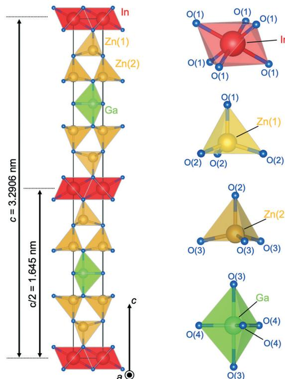
Fig. 9 Crystal structure of  $\text{InGaO}_3(\text{ZnO})_4$ . Coordination of  $\text{InO}_6$  octahedra,  $\text{Zn}(1)\text{O}_4$  tetrahedra,  $\text{Zn}(2)\text{O}_4$  tetrahedra, and  $\text{GaO}_5$  trigonal bipyramid.
