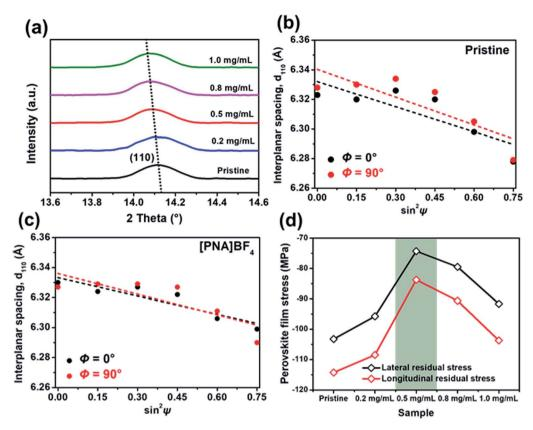
Fig. 3 (a) XRD spectra of magnified (110) lattice plane diffraction peaks for perovskite films grown on PEDOT:PSS and different concentrations of the [PNA]BF<sub>4</sub> layer; XRD  $d_{110}$  versus  $\sin^2 \psi$  plots for perovskite film grown on (b) PEDOT:PSS and (c) [PNA]BF<sub>4</sub> layer (5 mg mL<sup>-1</sup>); (d) lateral and longitude residual stress (or strain) of perovskite films based on PEDOT:PSS and different concentration [PNA]BF<sub>4</sub> layer.
