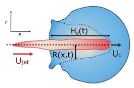
Fig. 4 Diagram illustrating the parameters used in this section. The jet impacts the pendant droplet from the left with velocity  $U_{\rm jet}$ , creating a cavity with increasing depth in time  $H_c(t)$ , where the velocity of the apex of the cavity is indicated by  $U_c = \dot{H}_c$  and whose radius depends on time and the position R(x, t). Here, x is the direction along which the jet travels and r is its perpendicular radial direction.
