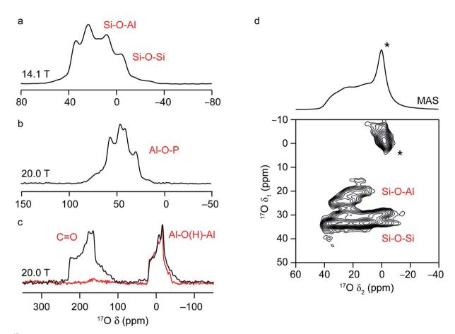
Fig. 3 17O MAS NMR spectra of (a) aluminosilicate CHA zeolite, (b) calcined CHA-type aluminophosphate framework, SIZ-4 and (c) calcined Al-MIL-53. The external field strengths at which spectra were recorded are shown in the figure. In (c), the  $^{1}H-^{17}O$  CP MAS NMR spectrum is shown in red. (d) <sup>17</sup>O (14.1 T) MAS and MQMAS of a hydrated CHA zeolite (after slurrying with H<sub>2</sub><sup>17</sup>O(l)).
