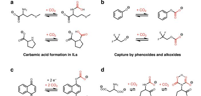
Fig. 2 New  $CO_2$  absorption mechanisms in solution. (a) Proposed formation of carbamic acid in ILs with amine-functionalised anions.<sup>37</sup> (b) Proposed absorption mechanism by phenoxide and alkoxide ILs.<sup>38</sup> (c) Proposed mechanism for electrochemical  $CO_2$  capture by 1,4-naph-thoquinone.<sup>39</sup> (d) Proposed absorption mechanism for an IL with an aspartate dianion.<sup>40</sup> In all cases, the corresponding cations are omitted for clarity.
