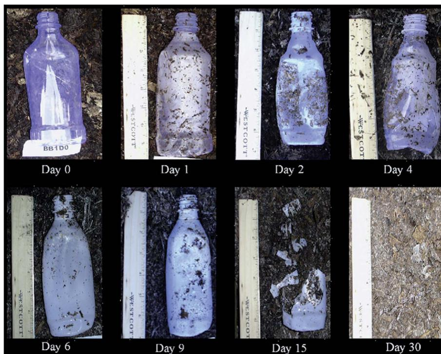
Fig. 28 PLA bottle biodegradation's chronology in the compost pile.<sup>101</sup>
