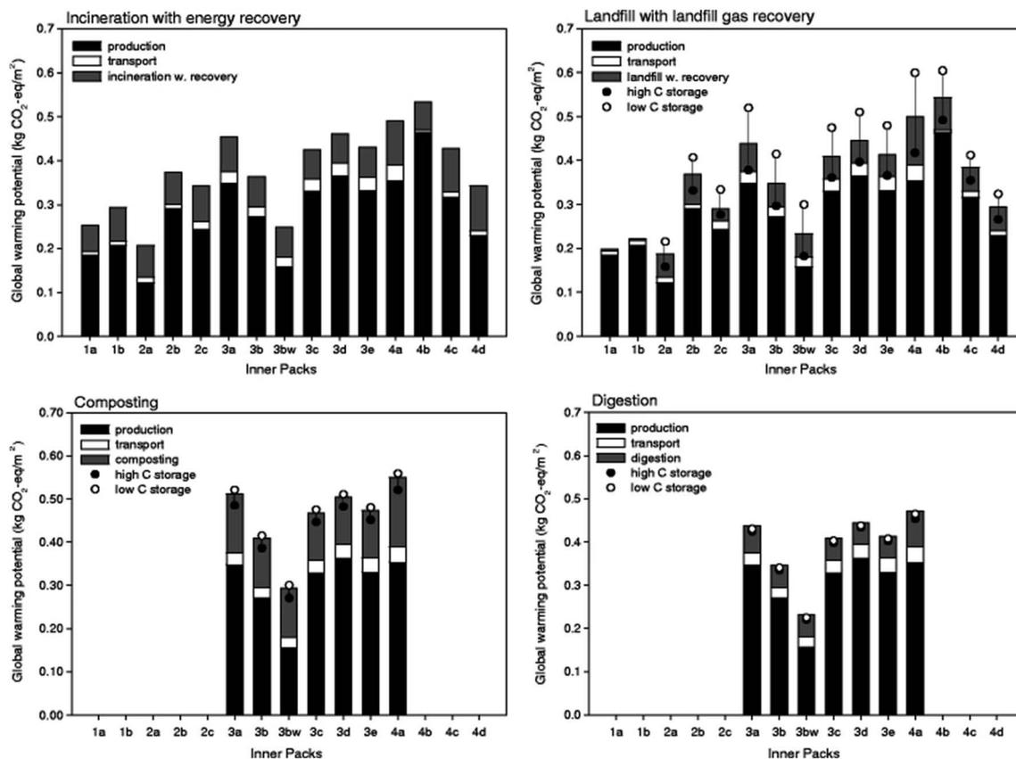
Fig. 33 Inner packs' global warming potential for four waste treatment types.<sup>117</sup>
