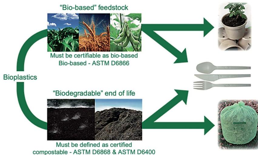
Fig. 4 Difference between bio based and biodegradable bioplastics.<sup>24</sup>
