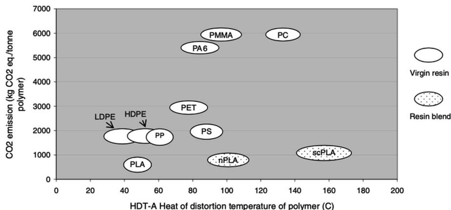
Fig. 32 Global warming potential of polymer production as a function of the heat distortion temperature of the polymer.<sup>115</sup>
