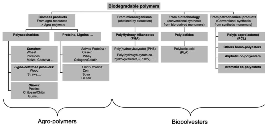
Fig. 14 Main biodegradable polymers classification.<sup>30</sup>
