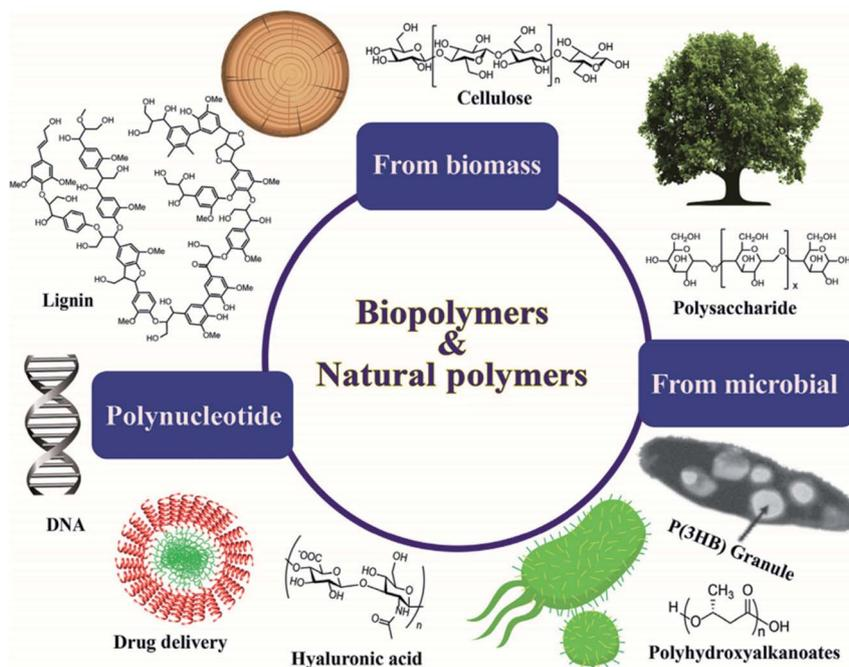
Fig. 7 Classifications of biopolymers based on their origins.<sup>26</sup>
