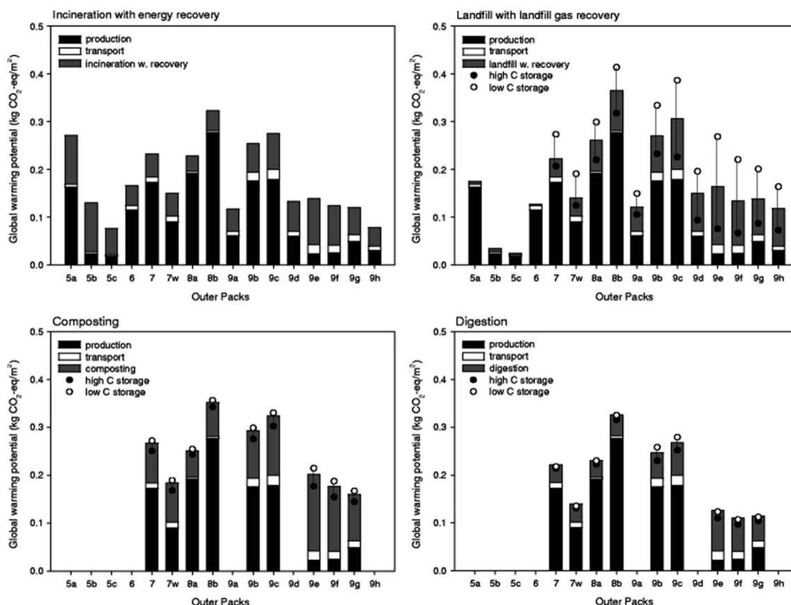
Fig. 34 Outer packs' global warming potential for four waste treatment types.<sup>117</sup>
