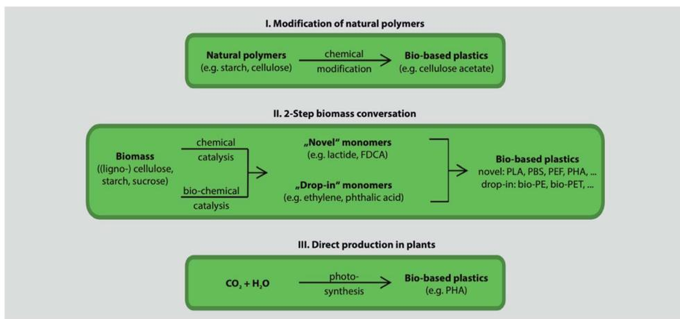
Fig. 12 The three main approaches to bio-based plastics.<sup>29</sup>
