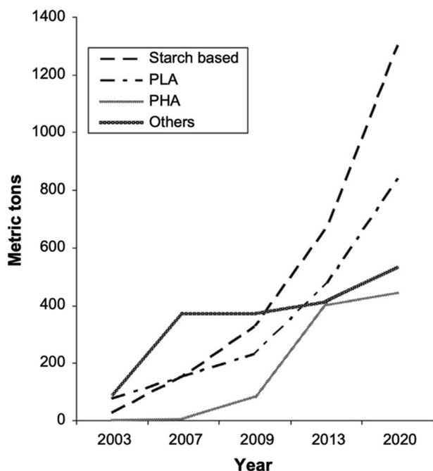
Fig. 18 Renewable biodegradable polymer's global production in 2003 to the projection for 2020.<sup>49</sup>
