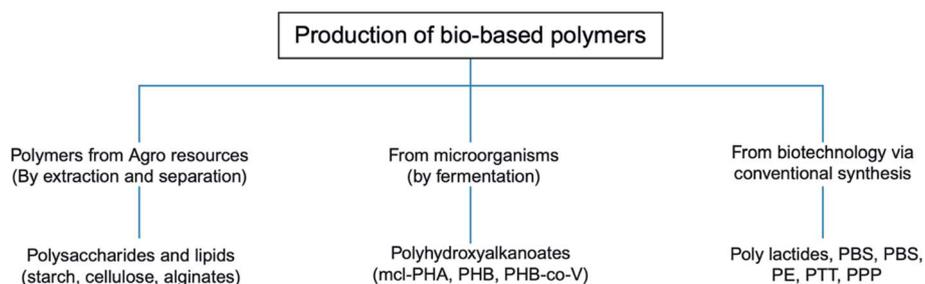
Fig. 13 The three main ways for the production of bio-based polymers.<sup>30,31</sup>
