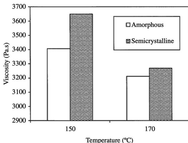
Fig. 21 Melt viscosity of semi crystalline and amorphous PLA at different temperatures.<sup>68</sup>
