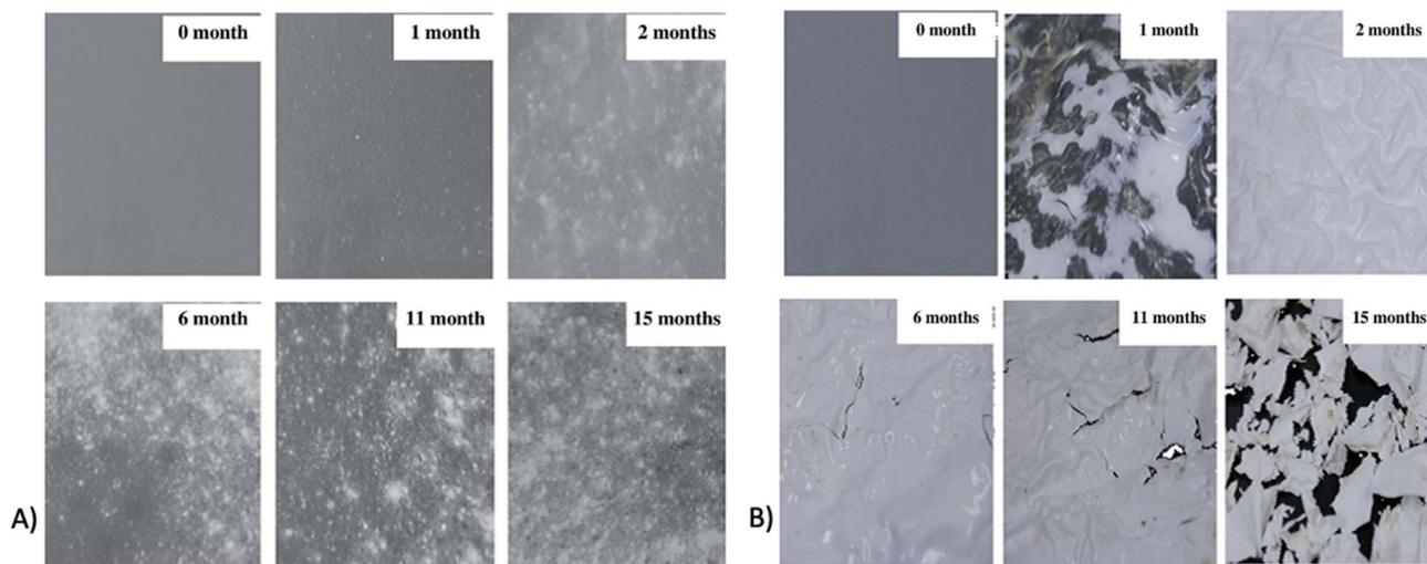
Fig. 29 PLA sheets' degradation under: (A) wastewater treatment condition, (B) landfills conditions.<sup>99</sup>
