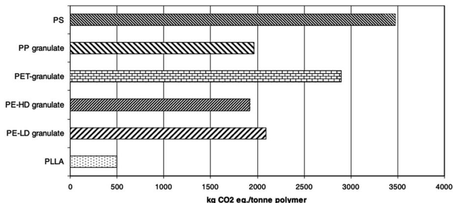
**Fig. 31** Global warming potential associated with the production of PLLA and other polymers.<sup>115</sup>
