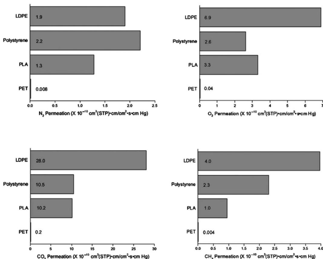
Fig. 25 Properties of permeation for 100% linear PLA with an L : D ratio 96 : 04 compared to other plastics commonly used for packaging at 30 °C.<sup>81</sup>
