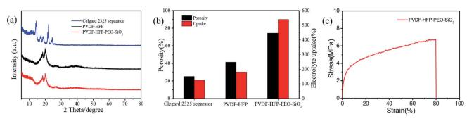
Fig. 3 (a) XRD patterns, (b) porosity and electrolyte uptake of the Celgard 2325 separator, pure PVDF-HFP and PVDF-HFP-PEO-SiO<sub>2</sub>, (c) stress-strain curve of the PVDF-HFP-PEO-SiO<sub>2</sub> GPE.
