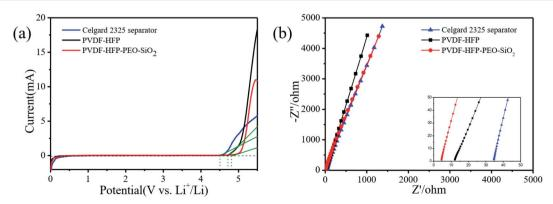
Fig. 4 (a) LSV curves and (b) impedance spectra of the Celqard 2325 separator absorbed liquid electrolyte and PVDF-HFP-based GPEs.
