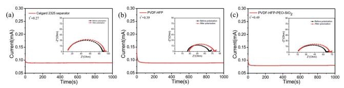
Fig. 5 Chronoamperometry curves of (a) Celgard 2325 separator, (b) PVDF-HFP, (c) PVDF-HFP-PEO-SiO<sub>2</sub> in the symmetrical Li/GPE/Li cells. AC impedances before and after polarization are shown in the inset.
