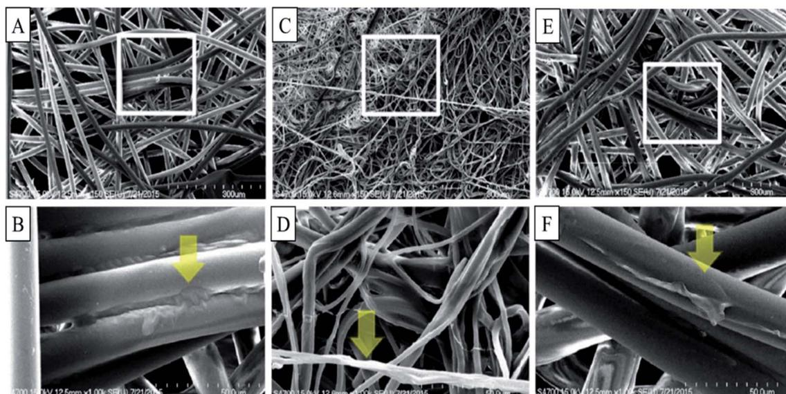
Fig. 10 SEM images: (A and B) first-layer; (C and D) second-layer; (E and F) third-layer of a commercial three-layered surgical mask coated with 1% GS5. (A), (C) and (E) have a magnification of 150 $\times$ . White boxes in (A), (C), and (E) is magnified by 1000 $\times$ , as shown in (B), (D), and (F). This figure is reproduced from ref. 100 with permission from Taylor & Francis, copyright 2016.
