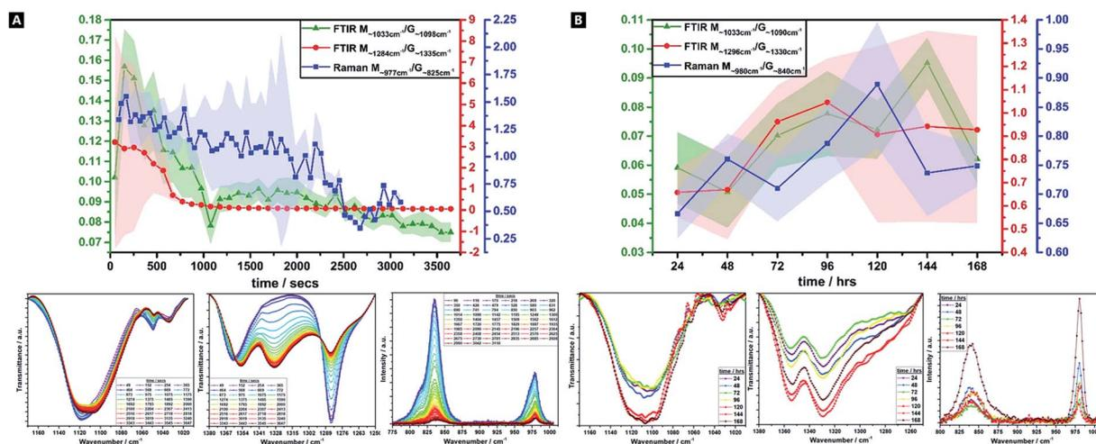
Fig. 4 Alginate M/G ratio variations over time as calculated from FTIR ( $1033 \text{ cm}^{-1}/1098 \text{ cm}^{-1}$  &  $1284 \text{ cm}^{-1}/1335 \text{ cm}^{-1}$ ) and Raman spectroscopy ( $977 \text{ cm}^{-1}/825 \text{ cm}^{-1}$ ) data, over the 60 minute (A) and 24–168 h ranges (B).
