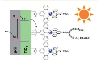
Fig. 10 Schematic diagram of p-Si|meso-TiO<sub>2</sub>|CotpyP photocathode used in photoelectrolytic reduction of CO<sub>2</sub>. 107
