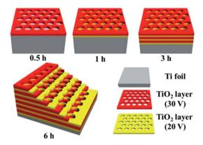
Fig. 5 Schematic diagram of titania photonic crystals prepared by anodisation and calcination of titanium foil. Image adapted with permission from ACS Publications.<sup>72</sup>
