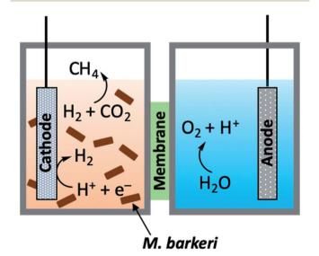
Fig. 13 General schematic diagram of hybrid bio-PEC cell. 118
