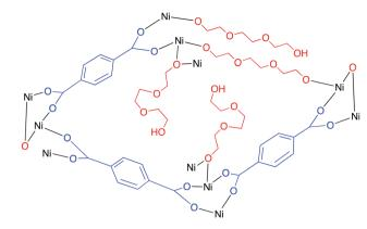
Fig. 21 Ni(TPA/TEG) composite formed for the heterogeneous photoconversion of carbon dioxide. Red organic linkers are TEG, and blue organics are TPA.<sup>169</sup>
