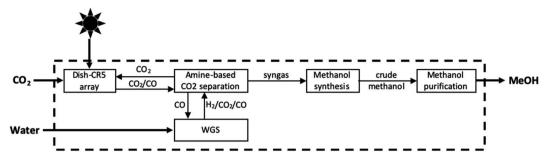
Fig. 9 Block flow diagram of photothermal conversion of  $CO_2$  to methanol by S2P process.<sup>84</sup>
