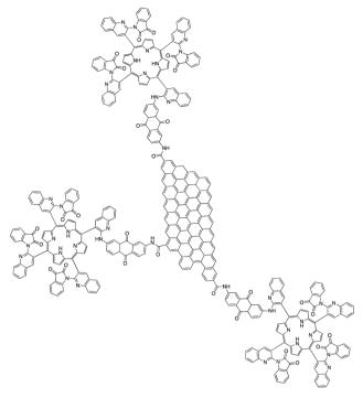
Fig. 24 CCG-IP photocatalyst used in photocatalytic/biocatalytic reduction of CO<sub>2</sub> to methanol. 183
