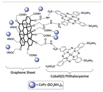
Fig. 22 Graphene-tethered cobalt(II) phthalocyanine catalyst for heterogeneous photoconversion of CO<sub>2</sub> to methanol. 174
