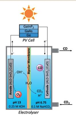
Fig. 11 Schematic diagram of modular photoelectrolyser used in carbon dioxide reduction mediated by bifunctional ALD-SnO<sub>2</sub>|CuO electrodes.109
