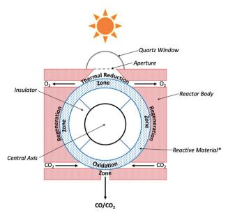
Fig. 8 Schematic diagram of CR5 used for CO2 photoconversion. \*Reactive material is comprised of sets of counter-rotating rings. Current cross-sectional view shows single ring oriented coincident with the plane of this page.83,84
