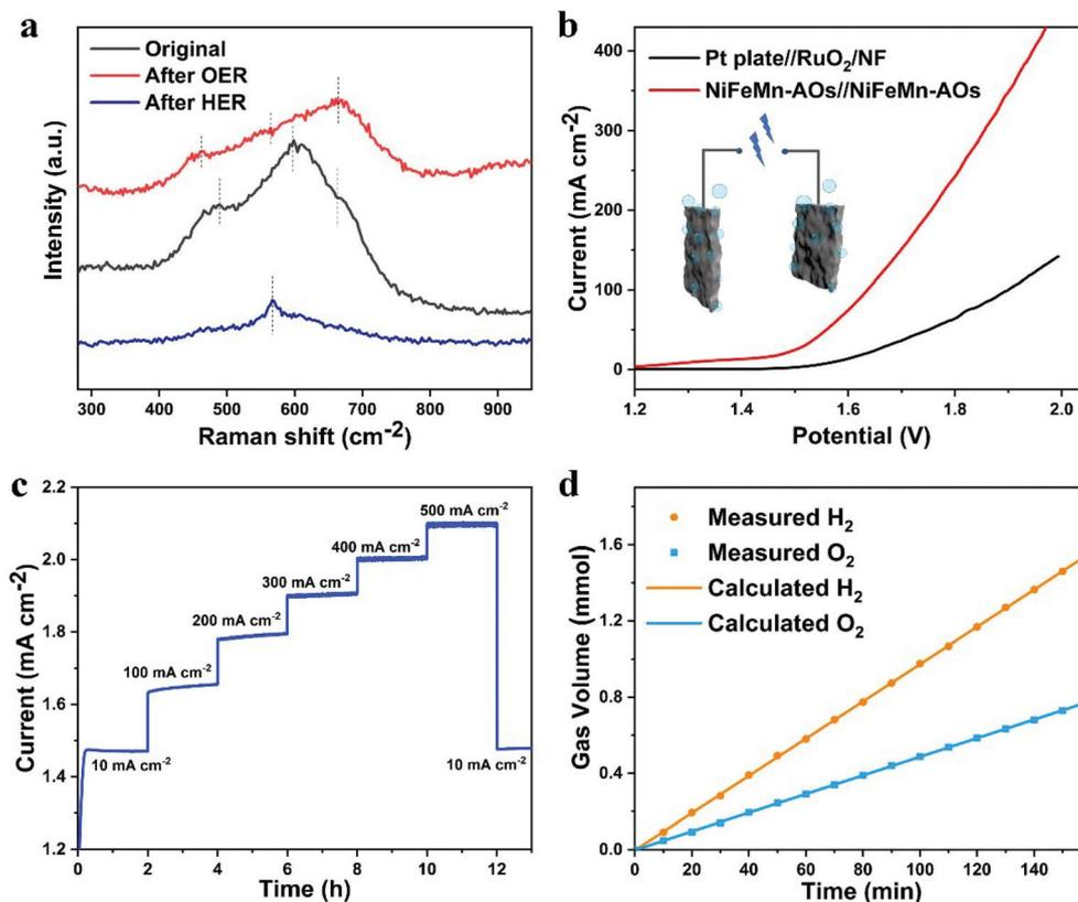
Fig. 5 (a) Raman spectra of the NiFeMn-AOs sample. (b) Polarization curves of NiFeMn-AOs//NiFeMn-AOs and Pt plate//RuO<sub>2</sub> electrolyzer (without iR-compensation). (c) Chronopotentiometry curves of NiFeMn-AOs//NiFeMn-AOs at various current densities. (d) The volumes of H<sub>2</sub> and O<sub>2</sub> experimentally measured at 100 mA cm<sup>-2</sup>.
