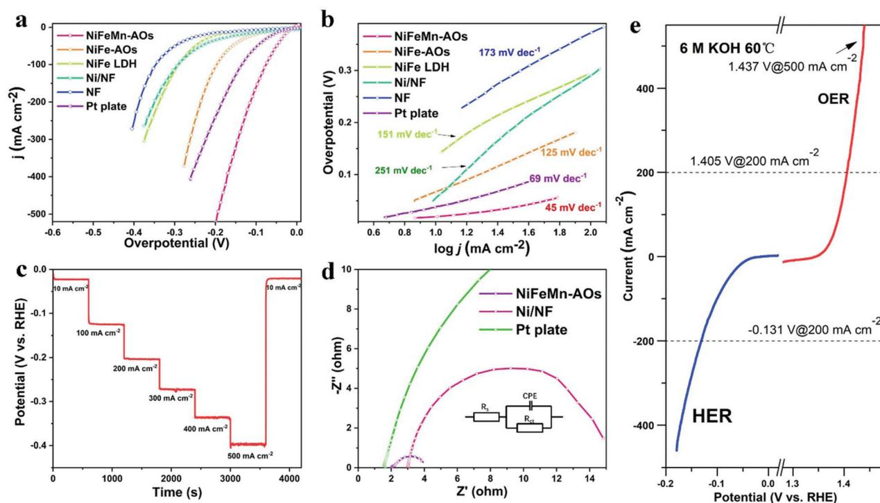
**Fig. 4** (a) The LSV curves of various electrodes. (b) The Tafel plots calculated from LSV curves. (c) Multi-chronopotentiometry curves of NiFeMn-AOs at different current densities. (d) EIS Nyquist plots of the Pt plate, Ni/NF and NiFeMn-AOs electrodes with 150 mV overpotential for HER. (e) HER and OER polarization curve of electrode NiFeMn-AOs under industrial operating conditions of 6 M KOH, 60 °C.
