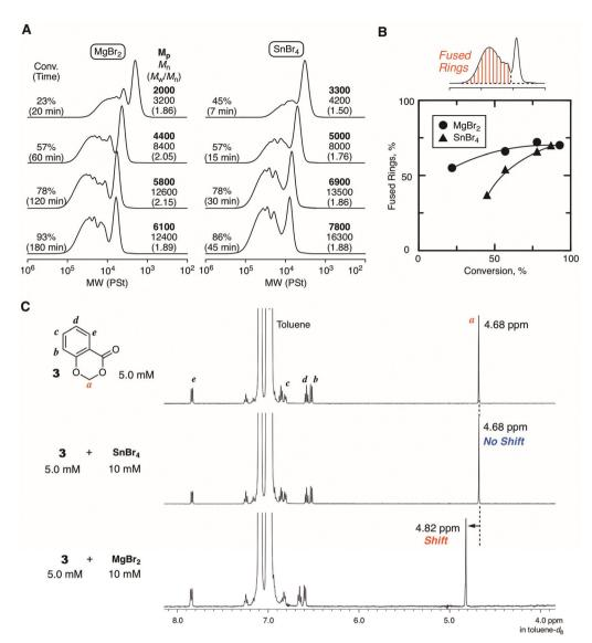
Fig. 4 Comparison between MgBr<sub>2</sub> and SnBr<sub>4</sub> in the ring-expansion cationic polymerization of IBVE with 1: (A) SEC curves of the obtained poly (IBVE)s (B) ratios of the fused ring estimated by peak separation. (C) <sup>1</sup>H NMR analyses of the mixture of MgBr<sub>2</sub> or SnBr<sub>4</sub> with 3 as the model compound for the evaluation of the interaction with the HAE bond.
