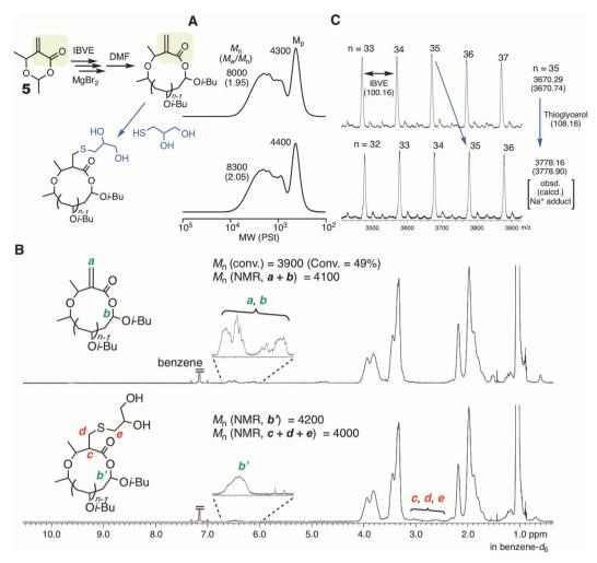
Fig. 6 Ring-expansion cationic polymerization of IBVE with 5 and MgBr<sub>2</sub>, and the post-polymerization reaction of the vinylidene group with thioglycerol. (A) SEC; (B)  $^{1}H$  NMR; (C): MALDI-TOF-MS [IBVE] $_{0}$ /[5] $_{0}$ /[MgBr $_{2}$ ] $_{0}$ /[DTBMP] $_{0}$  = 380/5.0/5.0 or 10/0.15 mM in toluene/Et $_{2}$ O (90/10 vol%) at 0 °C. The sample was obtained at 49% conversion (1 hour). See the ESI† for the conditions of the post-polymerization reaction.
