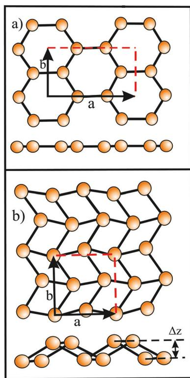
Fig. 6 (a) Honeycomb graphene-like lattice of gallene obtained by cleaving bulk  $\alpha$ -Ga along the (100) direction after relaxation ( $a_{100}$ -Ga). (b) Distorted rhombic lattice of gallene obtained by cleaving bulk  $\alpha$ -Ga along the (010) direction after relaxation ( $b_{010}$ -Ga). The dashed rectangle and square show the unit cells.
