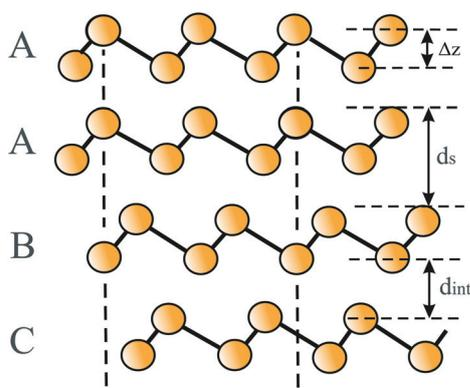
**Fig. 15** The stacking orders AA, AB, and AC of bilayers of buckled hexagonal monolayers. This figure defines the buckling effect  $\Delta z$ , the interlayer spacing  $d_s$ , and the distance between adjacent layers  $d_{int}$ .
