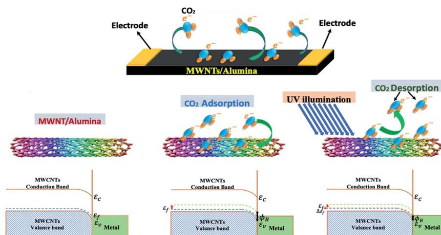
Fig. 8 Schematic representation of electron transfer on CNT surface and energy band diagram<sup>116</sup> (reprinted from ref. 116, Copyright (2017), with permission from Elsevier).
