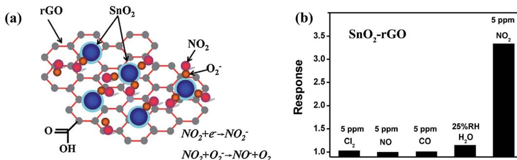
Fig. 7 (a) Illustration of the sensing mechanism for the gas sensor based on SnO<sub>2</sub>/rGO nanohybrid. (b) Selectivity (calculated using  $R_g/R_a$ ) histogram of SnO<sub>2</sub>/rGO gas sensor to various gases at room temperature.<sup>98</sup> (reprinted from ref. 98, Copyright (2014), with permission from Elsevier).
