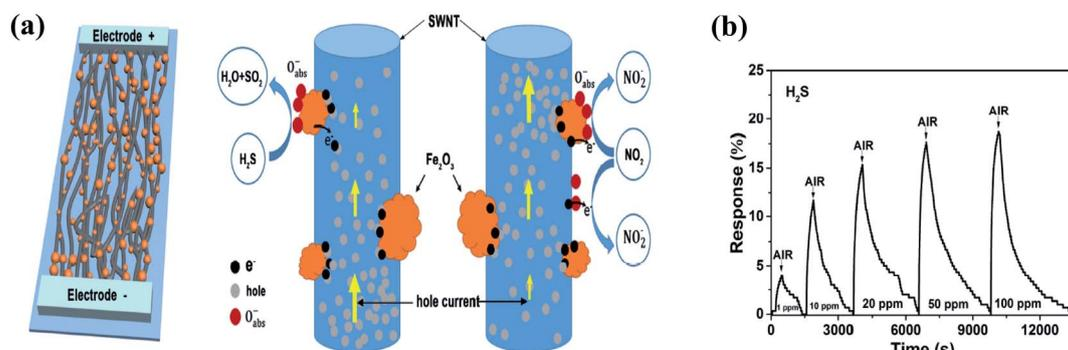
Fig. 15 (a) Schematic of the gas sensor based on SWNT- $\text{Fe}_2\text{O}_3$  composite film and schematic explaining the  $\text{H}_2\text{S}$  sensing mechanism. (b) Response ( $\Delta R/R_a$ ) and recovery curves of sensor upon exposure to  $\text{H}_2\text{S}$  (1, 10, 20, 50, and 100 ppm) with complete recovery<sup>107</sup> (reprinted from ref. 107. Copyright (2017), with permission from Elsevier).
