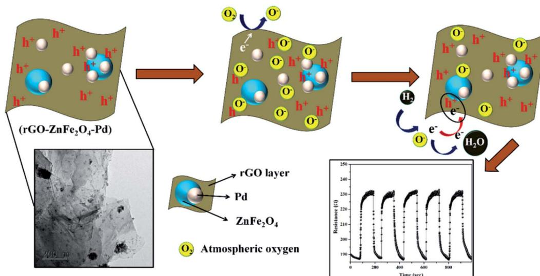
Fig. 14 Plausible sensing mechanism of  $\text{ZnFe}_2\text{O}_4$ -Pd decorated rGO towards  $\text{H}_2$  gas<sup>190</sup> (reprinted from ref. 190. Copyright (2020), with permission from Elsevier).
