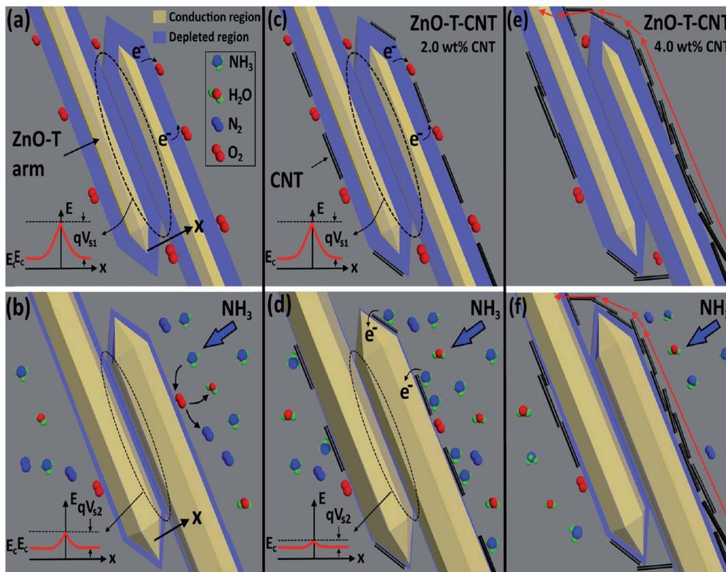
Fig. 10 Illustration of sensor in air (a) ZnO-T, (c) ZnO-T-2 wt% CNT networks and (e) ZnO-T-4 wt% CNT networks and in  $\text{NH}_3$  atmosphere (b) ZnO-T, (d) ZnO-T-2 wt% CNT networks and (f) ZnO-T-4 wt% CNT networks<sup>155</sup> (reprinted with permission from ref. 155. Copyright (2017) American Chemical Society).
