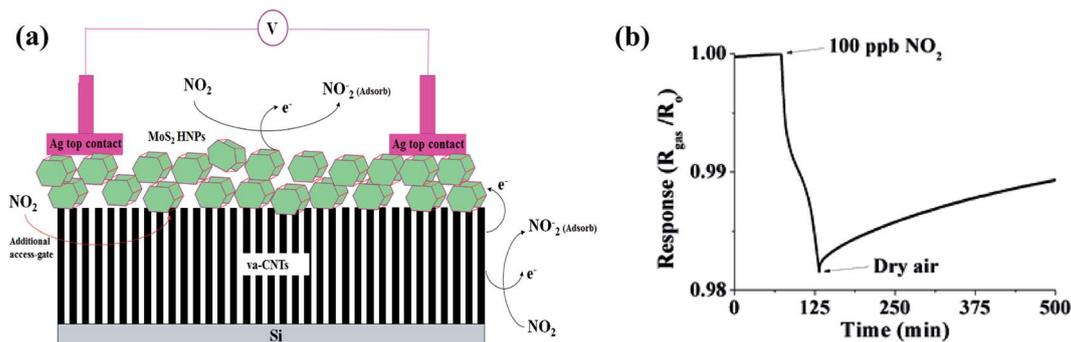
Fig. 6 (a) Schematic explaining the sensing mechanism of MoS<sub>2</sub> hexagonal nanoparticles (HNPs) on vertically aligned CNT array-based sensor. (b) Response of sensor at 100 ppb NO<sub>2</sub> gas<sup>34</sup> (reprinted with permission from ref. 34. Copyright (2017), John Wiley and Sons).
