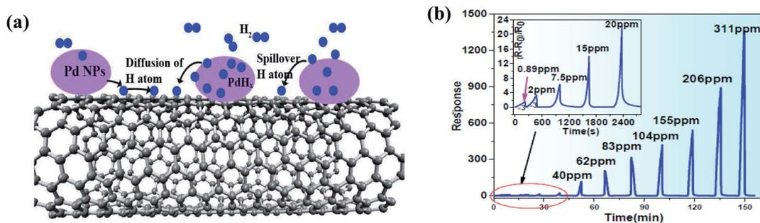
Fig. 13 (a) Schematic of H<sub>2</sub>-Pd-CNT interaction on CNT surface. (b) Response to different H<sub>2</sub> concentrations at ambient temperature<sup>180</sup> (adopted with permission from ref. 180. Copyright (2018) American Chemical Society).
