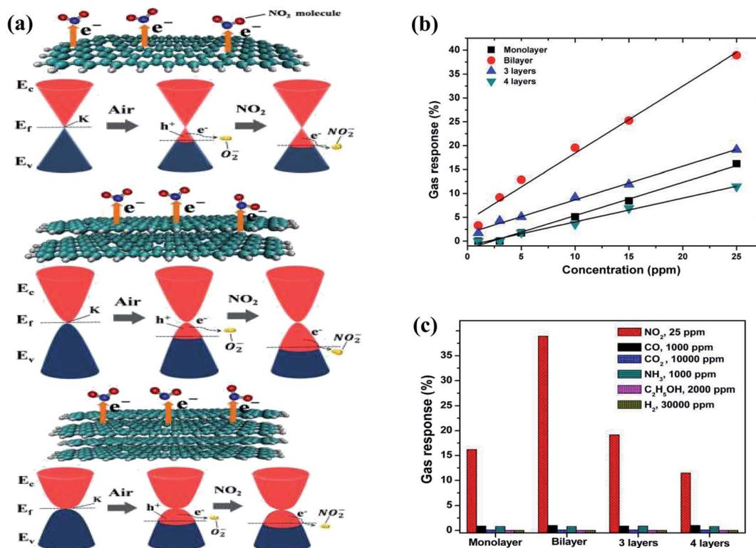
Fig. 5 (a) Schematic and band diagrams of  $\text{NO}_2$  sensing mechanism of monolayer, bilayer and multilayer graphene gas sensors. (b) Gas response ( $\Delta R/R$ ) of layered graphene gas sensors as a function of  $\text{NO}_2$  concentration. (c) Selectivity plot of layered graphene-based sensor to various gases at room temperature<sup>76</sup> (reprinted from ref. 76, Copyright (2017), with permission from Elsevier).
