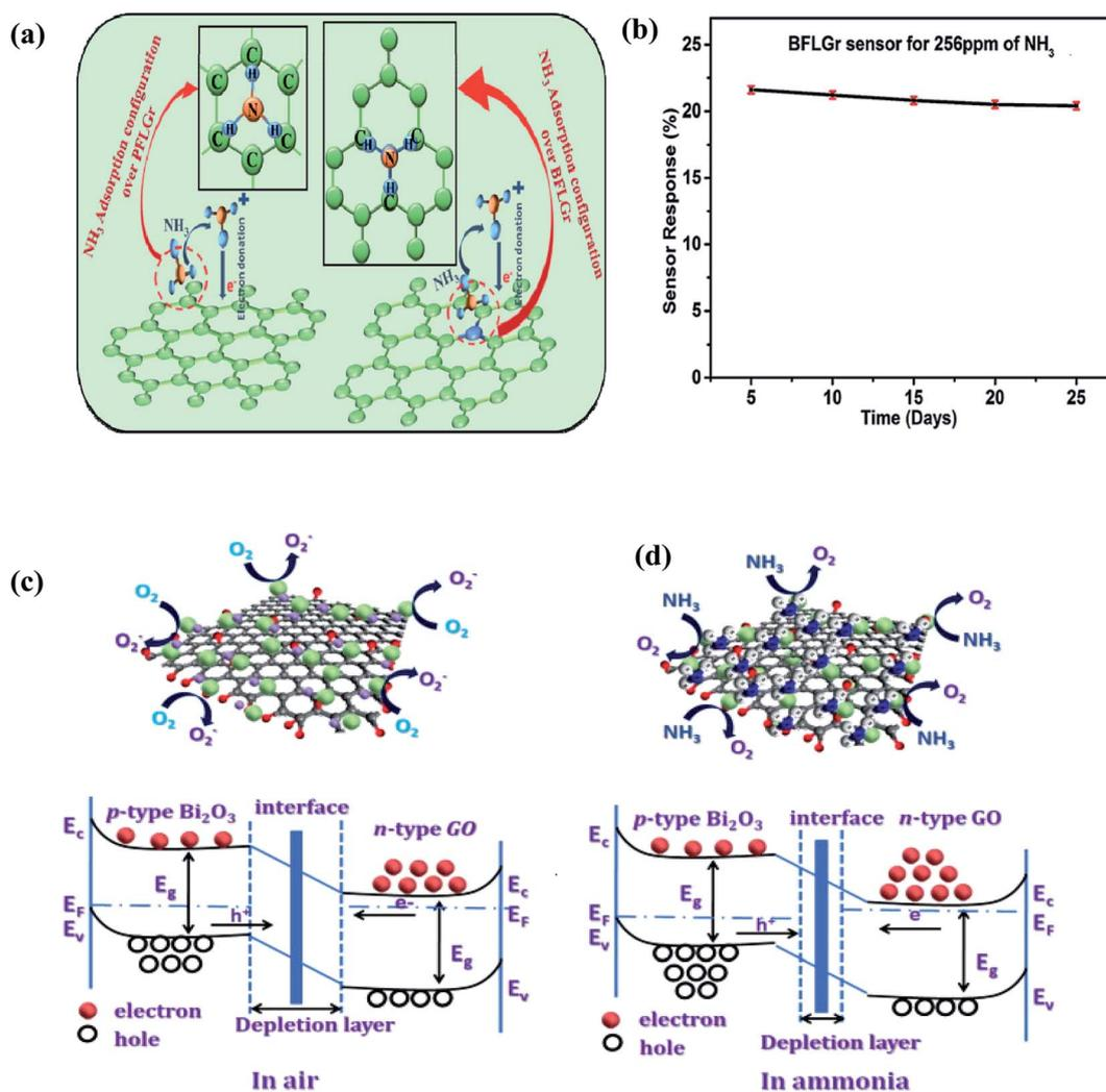
Fig. 12 (a) Schematic illustration of NH<sub>3</sub> adsorption and proposed gas sensing mechanism of the PFLGr and BFLGr sensor. (b) Plot of sensor response for a period of 25 days<sup>78</sup> (reprinted with permission from ref. 78. Copyright (2020), The Royal Society of Chemistry). Representation and band diagram of Bi<sub>2</sub>O<sub>3</sub>-doped graphene oxide in (c) air and (d) ammonia<sup>86</sup> (reprinted from ref. 86, Copyright (2021), with permission from Elsevier).
