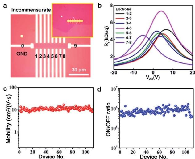
**Fig. 16** Performance of FETs based on the single-crystal 2D materials. (a) Optical micrographs of the bar-type patterned electrodes with GBs. (b) Sheet resistance between electrodes 0 and 9. (a and b) Reproduced with permission.<sup>18</sup> Copyright 2015, Wiley-VCH. (c and d) Carrier mobility and ON/OFF ratio of over 110 FETs. Reproduced with permission.<sup>87</sup> Copyright 2020, American Chemical Society.
