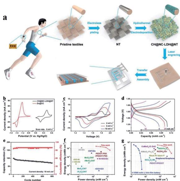
Fig. 2 (a) Fabrication process of Co-Zn alkaline microbattery. (b) Cyclic voltammograms of CH@NC-LDH@NT and Zn@CC at 5 mV s<sup>-1</sup>. (c) Cyclic voltammograms, (d) galvanostatic charge/discharge curves, (e) long-term cycling stability, and (f and g) Ragone plots of Co-Zn alkaline MB. Reproduced with permission.<sup>27</sup> Copyright 2020, Wiley-VCH.
