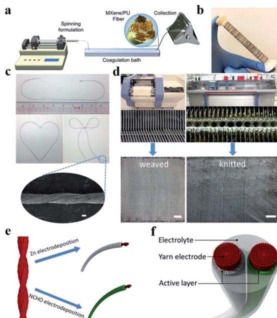
Fig. 7 (a) Schematic illustration of spinning process of the MXene/PU fiber. (b) Digital photograph of fabricated MXene/PU fiber. Reproduced with permission.<sup>120</sup> Copyright 2020, Wiley-VCH. (c) Flexibility demonstration and SEM image of the yarn. (d) Demonstration of weavability and knittability. (e) Schematics of yarns electrodeposited with Zn and NCHO and (f) solid-state yarn battery. Reproduced with permission.<sup>121</sup> Copyright 2017, American Chemical Society.
