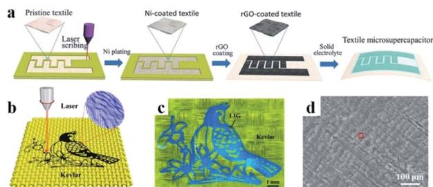
Fig. 3 (a) Fabrication process of textile MSCs. Reproduced with permission.<sup>16</sup> Copyright 2016, Wiley-VCH. (b) Schematic of the graphene/Kevlar textile from Kevlar. (c) SEM image of laser-induced graphene (LIG) on a Kevlar textile. (d) SEM image of the LIG circled in (b). Reproduced with permission.<sup>18</sup> Copyright 2020, American Chemical Society.
