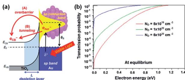
Fig. 8 (a) Band diagram picture of hot electron injection at the Au–TiO<sub>2</sub> heterojunction by (A) transfer over the barrier or (B) tunneling. Reproduced from ref. 96, copyright 2017, with permission from the Royal Society of Chemistry. (b) Tunneling probability at the Au–TiO<sub>2</sub> interface as a function of electron energy for different doping concentrations. Reprinted from ref. 90, copyright 2018, with permission from Elsevier.
