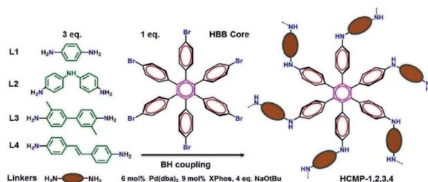
Fig. 14 Synthesis of hexaphenylbenzene-based CMPs. Adapted with permission.<sup>147</sup> Copyright 2016, American Chemical Society.
