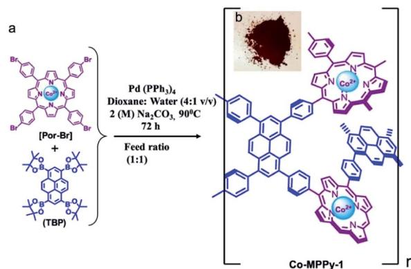
Fig. 3 Synthesis of metalloporphyrin and pyrene-based CMP, Co-MPPY-1. Adapted with permission.<sup>102</sup> Copyright 2019, American Chemical Society.
