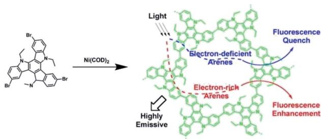
Fig. 15 Synthesis of carbazole-based CMP (TCB-CMP) and schematic of its sensing mechanism. Reproduced with permission.<sup>148</sup> Copyright 2012, American Chemical Society.
