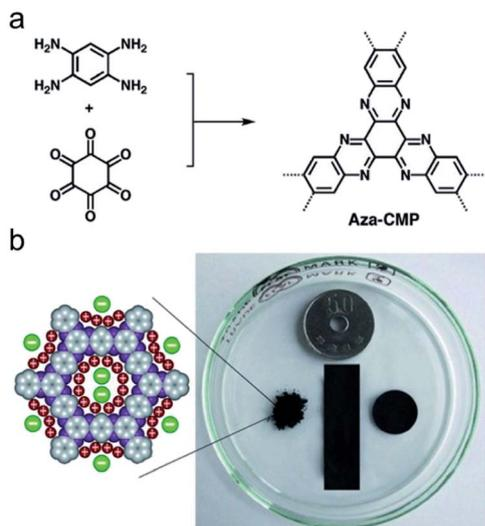
Fig. 5 (a) Synthesis of phenazine-fused aza-CMP and (b) schematic of enhanced electrolyte ions accumulation on the pore walls. Reproduced with permission.<sup>107</sup> Copyright 2013, John Wiley and Sons.
