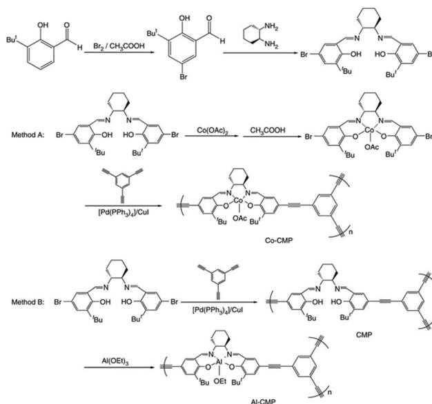
Fig. 4 Synthesis and metalation of Salen-based CMPs, Co-CMP, and Al-CMP. Adapted with permission.<sup>104</sup> Copyright 2013, Nature Publishing Group.
