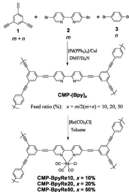
Fig. 6 Synthesis of metal-CMP *via* post-synthetic metalation. Adapted with permission.<sup>114</sup> Copyright 2010, John Wiley and Sons.
