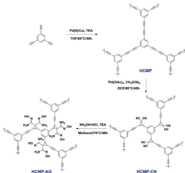
Fig. 9 Synthesis of HCMP-1 functionalized with bis-amidoxime groups. Adapted with permission.<sup>122</sup> Copyright 2020, American Chemical Society.
