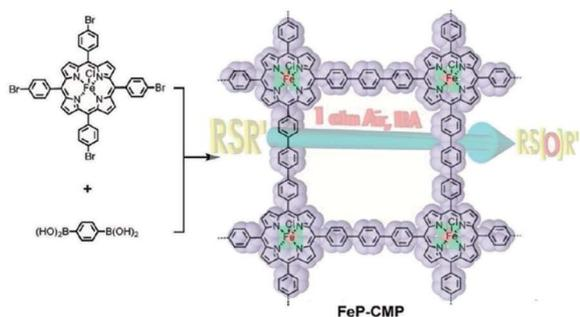
Fig. 11 Synthesis of the nano-heterogeneous catalyst with metal-loporphyrin built-in skeleton (FeP-CMP). Reproduced with permission.<sup>112</sup> Copyright 2010, American Chemical Society.
