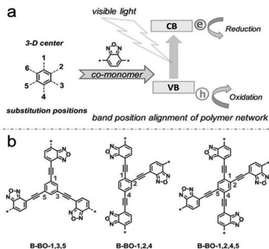
Fig. 12 (a) Geometry design principle of valence and conduction band position modification. (b) Synthesis of CMPs with the substitution position modification. Reproduced with permission.<sup>139</sup> Copyright 2015, John Wiley and Sons.
