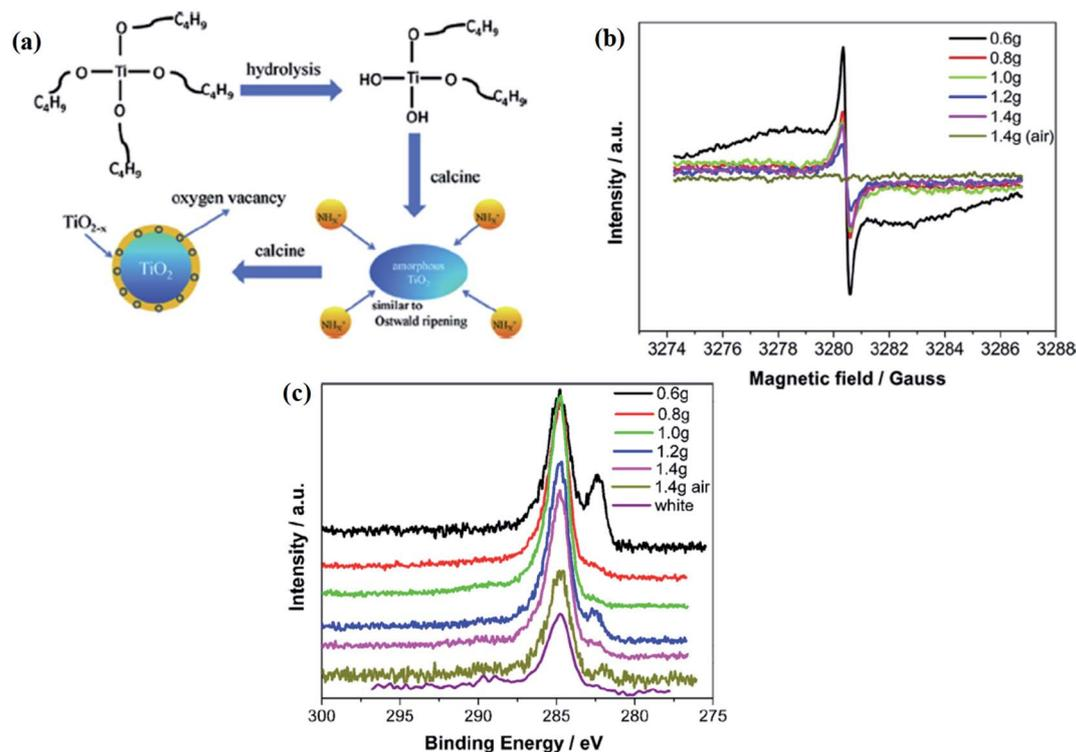
Fig. 7 (a) Schematic representations of the formation mechanism of  $\text{TiO}_2@\text{TiO}_{2-x}$ , (b) EPR spectra, (c) C 1s XPS analysis of the white, black and yellow  $\text{TiO}_2$  after 60 s  $\text{Ar}^+$  etching. Reprinted with permission from ref. 73. Copyright 2016 Elsevier.
