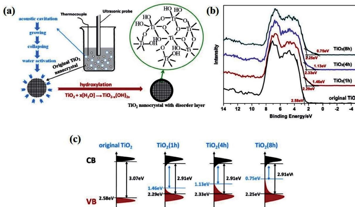
Fig. 13 (a) Schematic representations of the surface disorders generated by the ultrasonication process, (b) VB XPS plot of the parent and  $\text{TiO}_2$  nanocrystals after ultrasonication, and (c) the energy profile diagram of the material for different time periods of ultrasonic treatment. Reprinted with permission from ref. 90. Copyright 2017 Elsevier.
