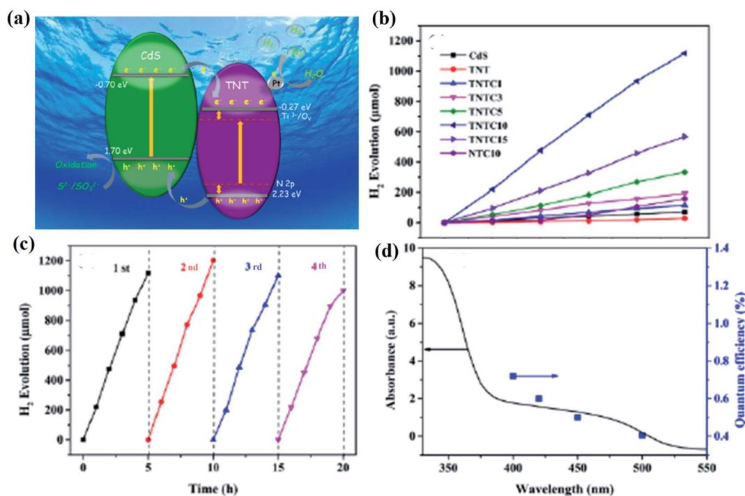
Fig. 23 (a) Mechanism of hydrogen production by the composite TNTNC10, (b) photocatalytic hydrogen generation rate by various samples, (c) reusability of the H-TiO<sub>2</sub> composite, and (d) wavelength-dependent AQE of hydrogen evolution. Reprinted with permission from ref. 107. Copyright 2019 Elsevier.
