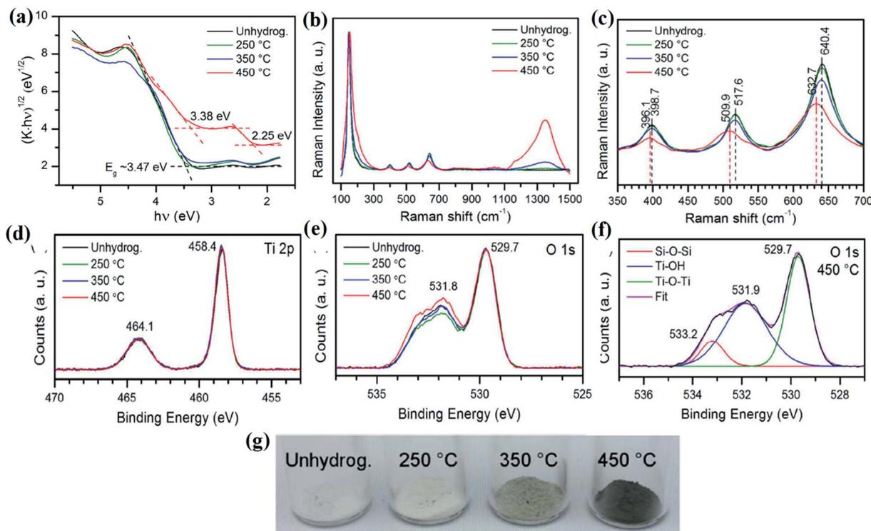
Fig. 1 (a) UV-Vis DRS, (b and c) Raman, and (d–f) XPS spectra of H-TiO<sub>2</sub>. Reprinted with permission from ref. 60. Copyright 2012, American Chemical Society.
