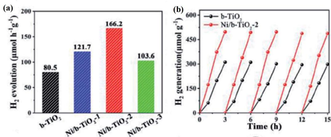
Fig. 22 (a) Photocatalytic hydrogen generation rate by B- $TiO_2$ , Ni/B- $TiO_2$ -1, Ni/B- $TiO_2$ -2, Ni/B- $TiO_2$ -3, and (b) the reusability of the non-noble metal co-catalyzed B- $TiO_2$ . Reprinted with permission from ref. 105. Copyright 2020 Elsevier.
