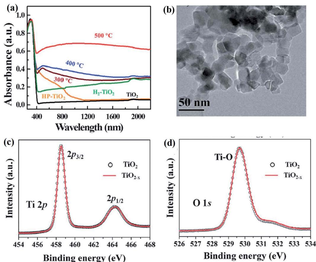
Fig. 8 (a) Absorbance spectra of the TiO<sub>2</sub> reduced at different temperatures, (b) TEM image of reduced TiO<sub>2</sub>, (c and d) XPS spectra (Ti 2p and O 1s) of the parent and reduced TiO<sub>2</sub>. Reprinted with permission from ref. 77. Copyright 2013, Royal Society of Chemistry.
