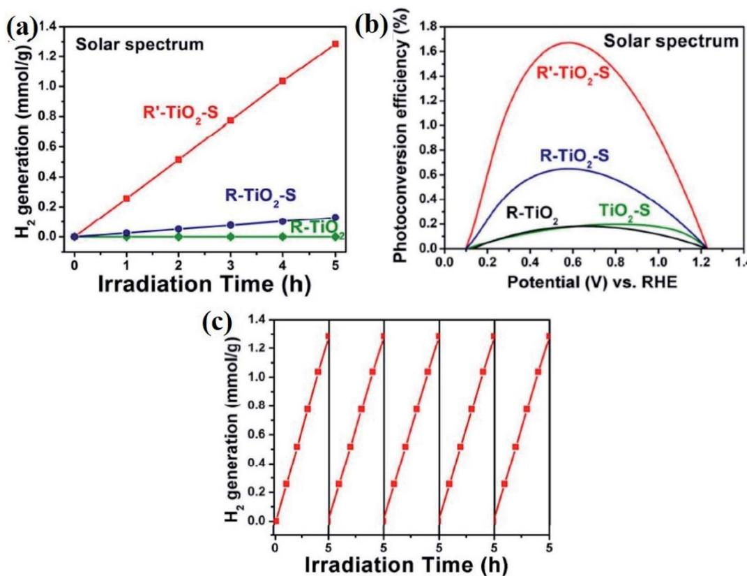
Fig. 17 (a) Visible light-driven hydrogen generation rate of various doped TiO<sub>2</sub>, (b) photoconversion efficiency of various S-doped photocatalysts, and (c) stability data of the photocatalyst. Reprinted with permission from ref. 99. Copyright 2013, American Chemical Society.
