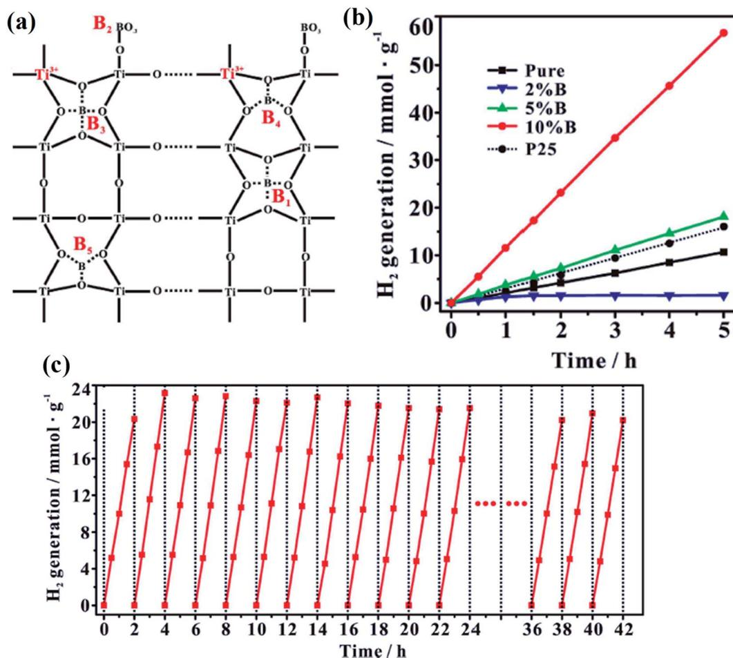
Fig. 19 (a) Schematic illustrations of the boron sites, (b) photocatalytic activity, and (c) reusability test graph of 10% boron doped TiO<sub>2</sub>. Reprinted with permission from ref. 101. Copyright 2016 Nature Journal.
