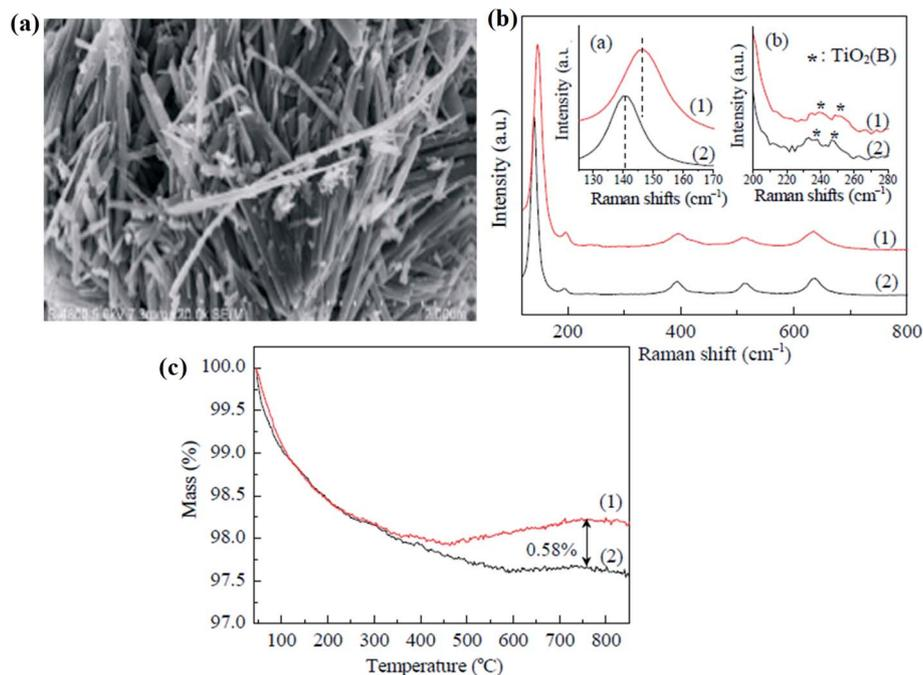
Fig. 4 (a) FESEM image of the H-TiO<sub>2</sub> nanofibers, (b) Raman spectra of the pristine and H-bicrystalline TiO<sub>2</sub>, and (c) TGA plot of the pure and H-TiO<sub>2</sub> nanofibers. Reprinted with permission from ref. 67. Copyright 2015 Elsevier.
