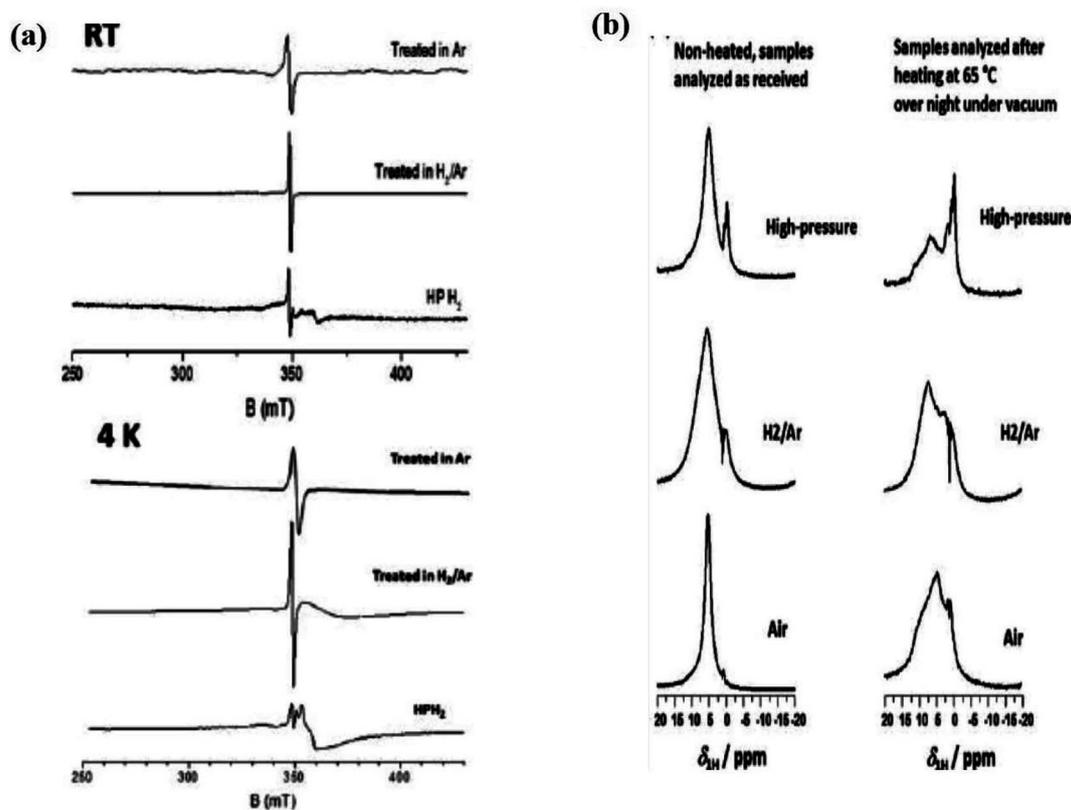
Fig. 3 (a) EPR data and (b) NMR spectra of the TiO<sub>2</sub> nanotube annealed in different atmospheric conditions (H<sub>2</sub>, Ar/H<sub>2</sub> and high pressure H<sub>2</sub>). Reprinted with permission from ref. 66. Copyright 2016, Royal Society of Chemistry.
