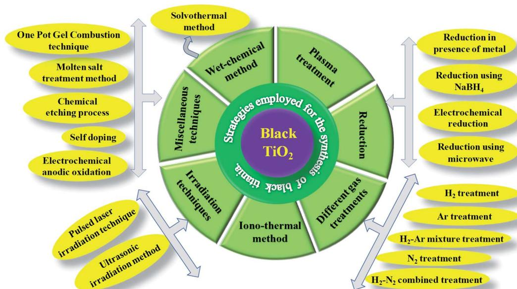
Scheme 1 Different preparation techniques adopted for fabricating B-TiO<sub>2</sub>.
