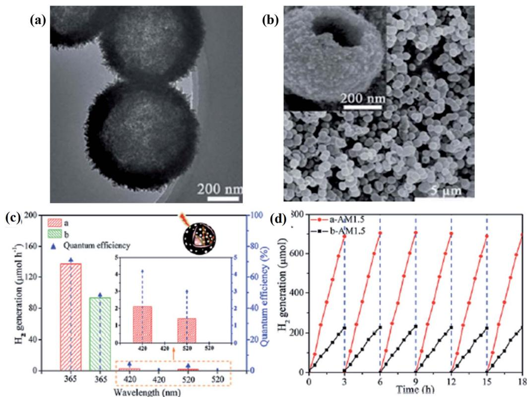
Fig. 24 (a) TEM image and (b) SEM image of the stable mesoporous B-TiO<sub>2</sub> hollow spheres, (c) photocatalytic hydrogen production rate by the mesoporous hollow spheres, and (d) cycling check for the stability of the mesoporous B-TiO<sub>2</sub> hollow sphere. Reprinted with permission from ref. 110. Copyright 2013, Royal Society of Chemistry.
