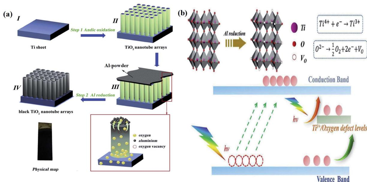
Fig. 15 (a) Schematic representations of the synthesis procedure of B-TiO<sub>2</sub> nanotube arrays, and (b) lattice structure of the material with its energy bands. Reprinted with permission from ref. 97. Copyright 2019 Elsevier.
