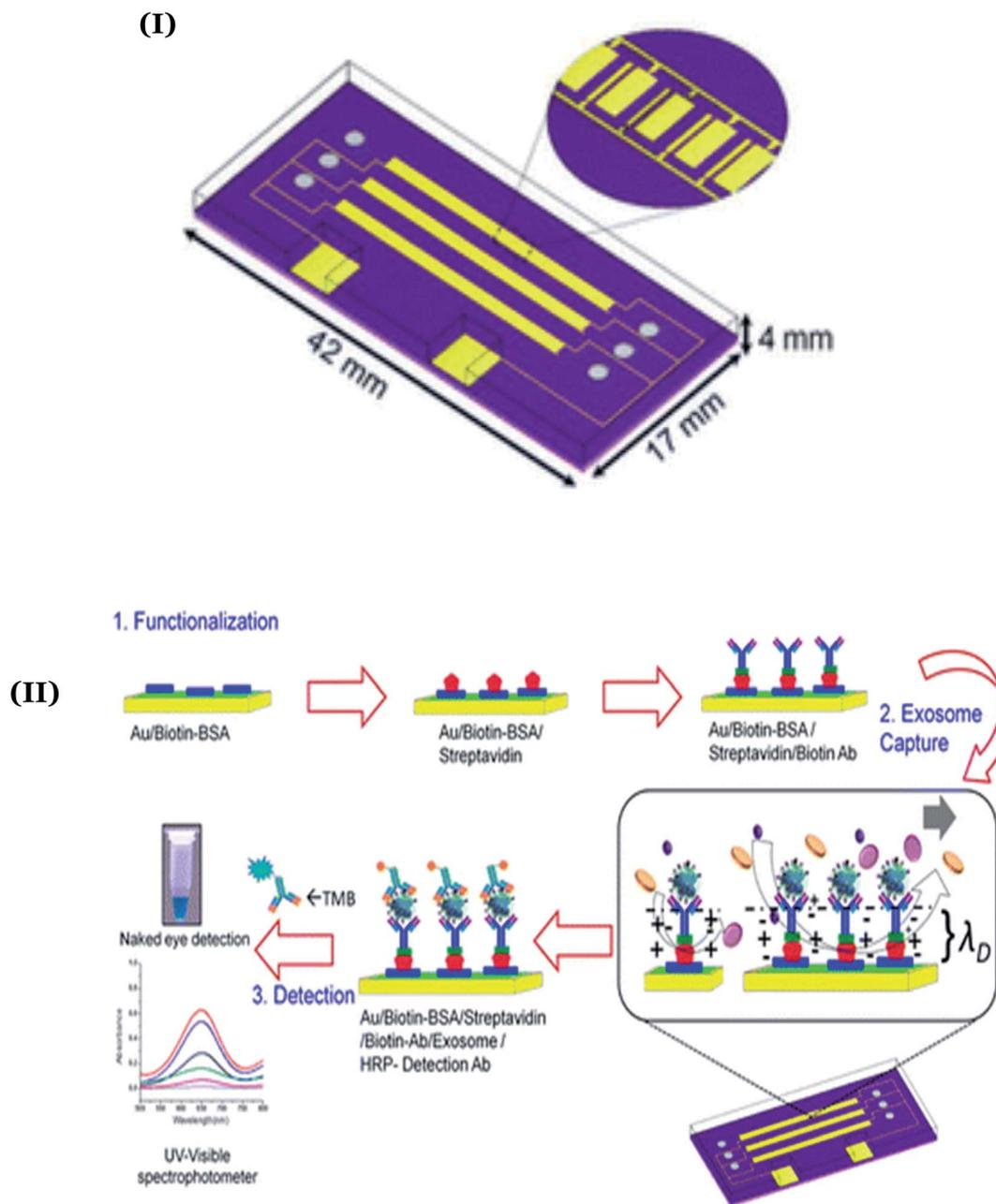
Fig. 7 (I) Design of the ac-EHD based multiplexed device for naked-eye detection of exosomes derived from HER2 positive cells. Adapted with permission.<sup>114</sup> Copyright 2014, American Chemical Society. (II) Detailed steps involved during the avidin-biotin assisted functionalization of the device with anti-HER2 and anti-CD9/anti-PSA. Reproduced with permission.<sup>114</sup> Copyright 2014, American Chemical Society.
