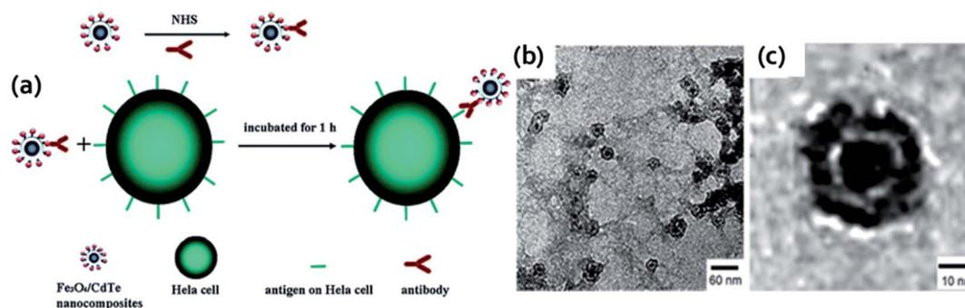
Fig. 6 (a) Schematic design of immuno-labeling by Fe<sub>3</sub>O<sub>4</sub>/CdTe nanocomposites. (b and c) TEM image of Fe<sub>3</sub>O<sub>4</sub>/CdTe MFNPs. Reproduced from ref. 2 with permission from American Chemical Society, copyright 2010.
