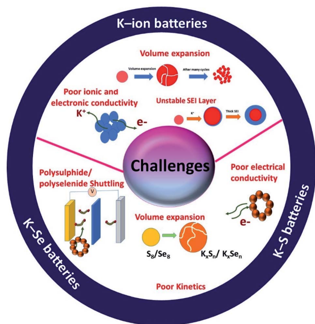
Fig. 3 Schematic of the challenges of potassium batteries.
