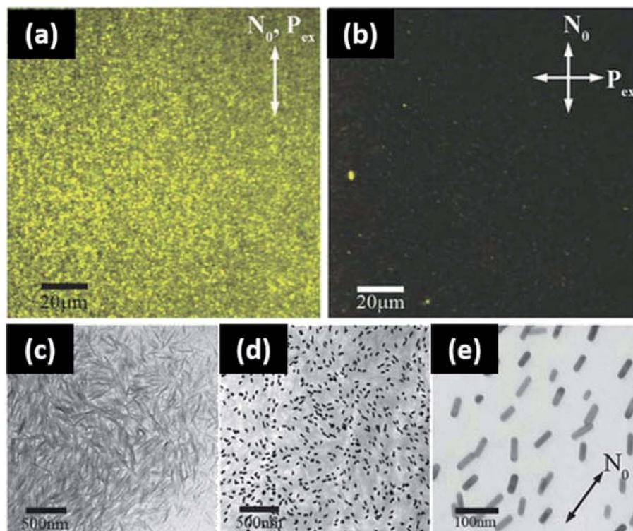
Fig. 13 Gold nanorod alignment in cellulose nanocrystal matrices for optoelectronic applications. Two-photon luminescence images of aligned gold nanorods in CNC with (a) the polarization excitation parallel to the aligned far field detector, (b) the polarization excitation perpendicular to the far field director, (c) TEM micrograph of CNCs alone, (d and e) TEM of aligned gold nanorods in CNCs. This figure was adapted from ref. 247, with permission from Wiley, 2014.
